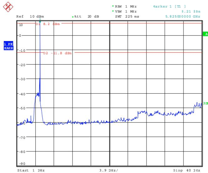
All emissions were at least 35 dB below the limit during the preliminary measurement, so no final measurement was carried out
