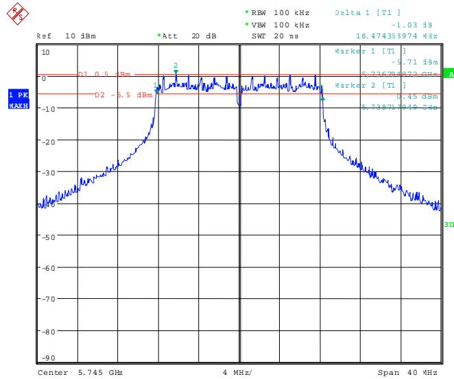
102732\_002.wmf: 6 dB bandwidth at the middle of the assigned frequency band, 9 Mbps:
