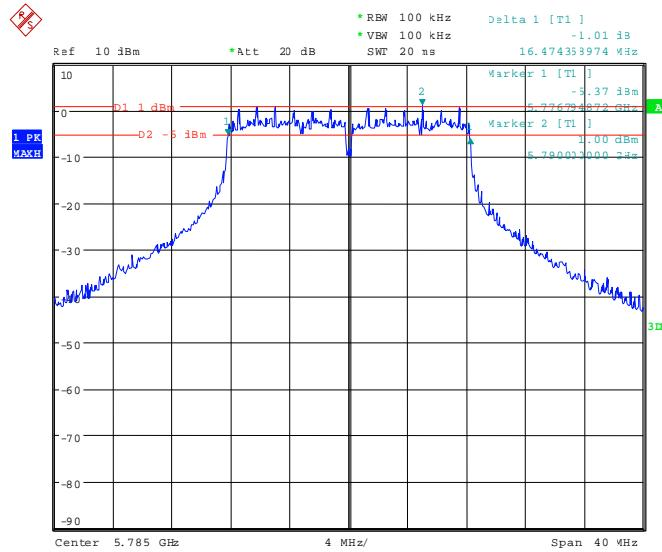
102732\_003.wmf: 6 dB bandwidth at the upper end of the assigned frequency band, 9 Mbps:
