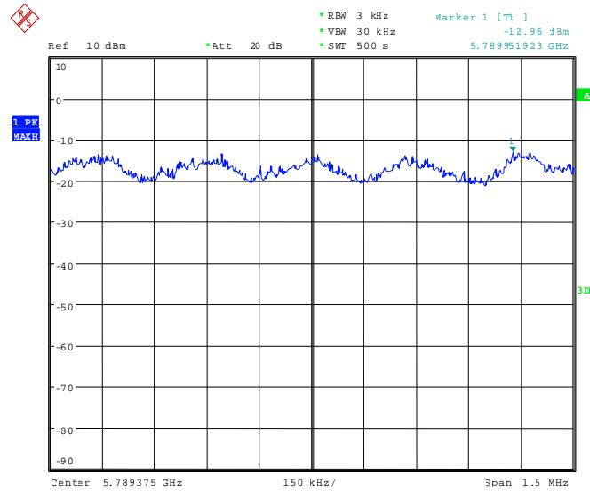
102732\_004.wmf: Power spectral density at the upper end of the assigned frequency band, 9 Mbps:
