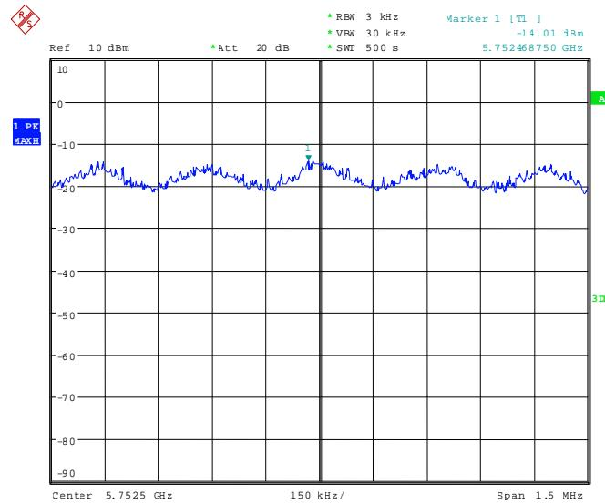
102732\_005.wmf: Power spectral density at the middle of the assigned frequency band, 9 Mbps:
