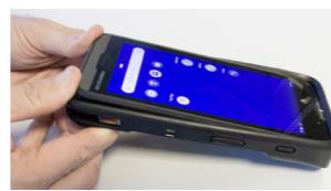
Insert the Memor 20 with the rubber boot into the dock with the screen facing front and the head facing up.
