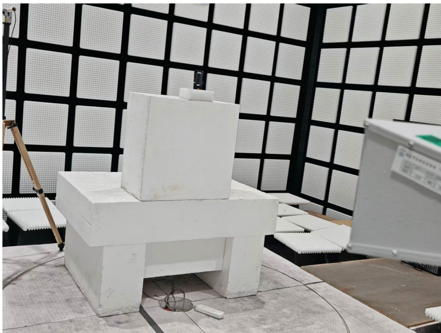
Description: Front view of Radiated Emission Test Setup (1GHz -18GHz)
