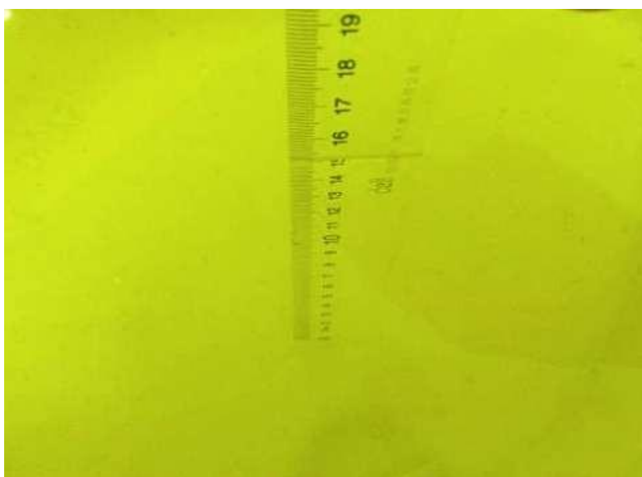
Picture 9.2-1: Liquid depth in the Flat Phantom
