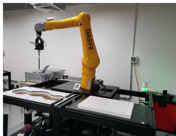
Picture D.6 Specific Absorption Rate Test Layout
