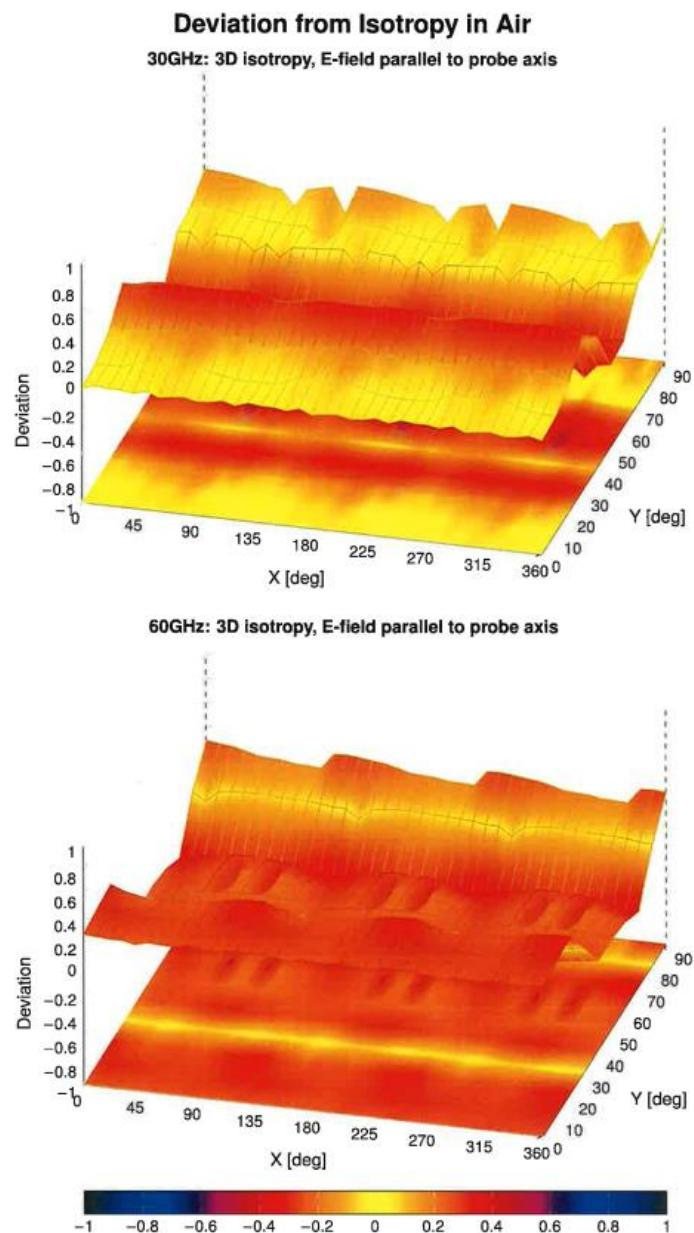
Probe isotropy for  $E_{tot}$ : probe rotated  $\phi = 0^\circ$  to  $360^\circ$ , tilted from field propagation direction  $\vec{k}$
