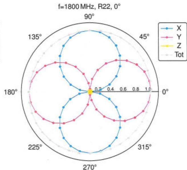
**Receiving Pattern ( $\phi$ ),  $\vartheta = 90^\circ$**
