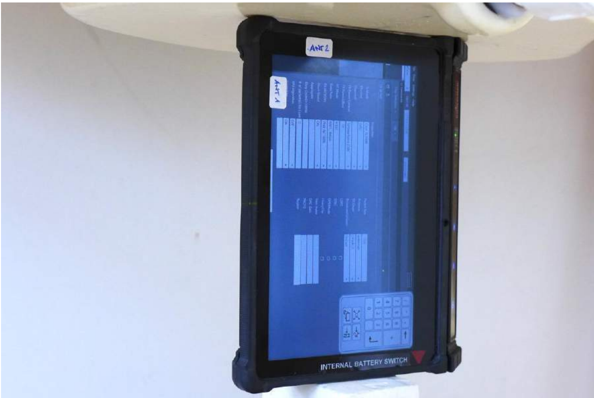
Pic. 5: Test position, edge 4 of DUT towards the phantom, 0 mm distance.
