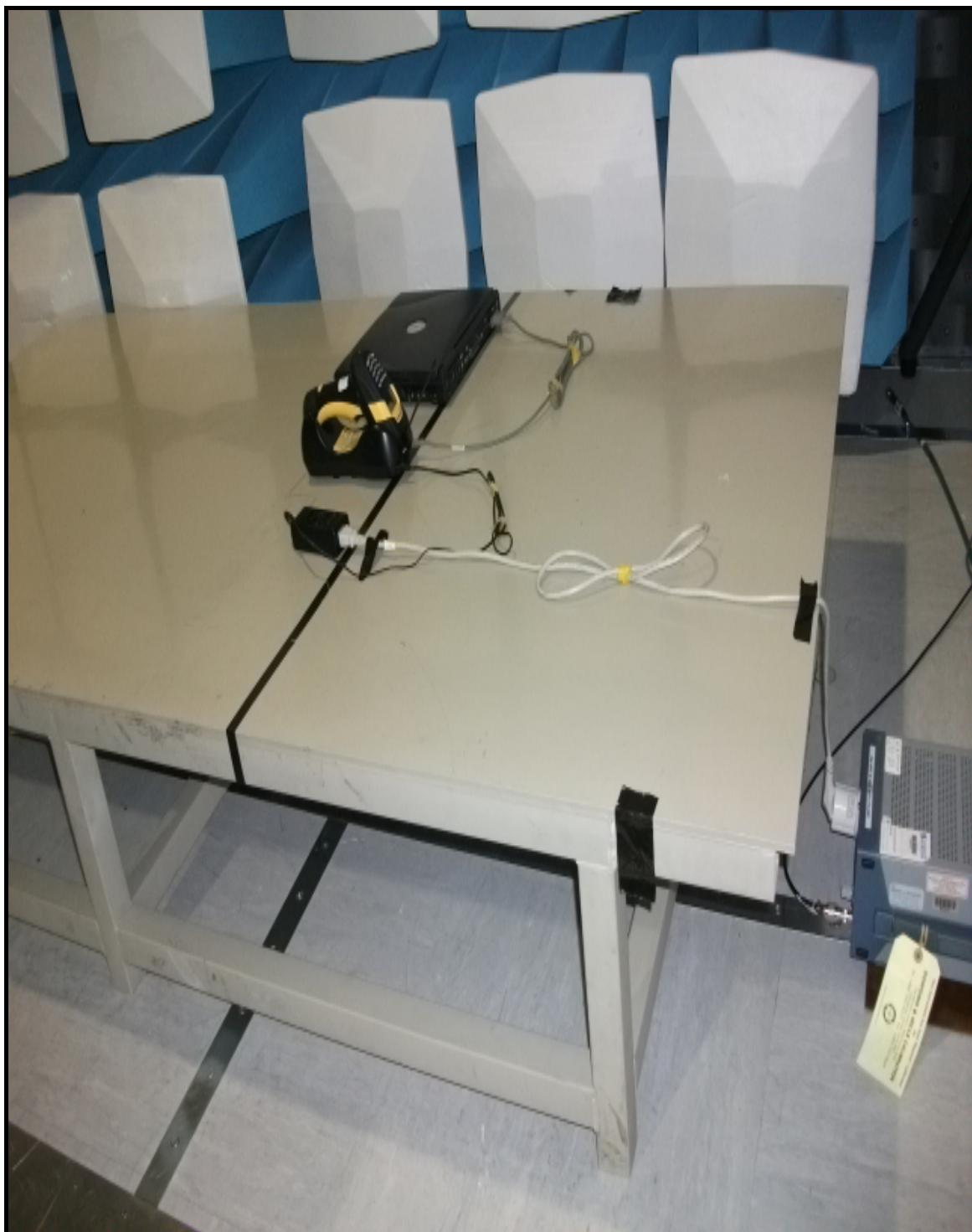
**PHT\77263JD03\002 - Test Configuration Photograph - Conducted Emissions (Out of cradle)**
