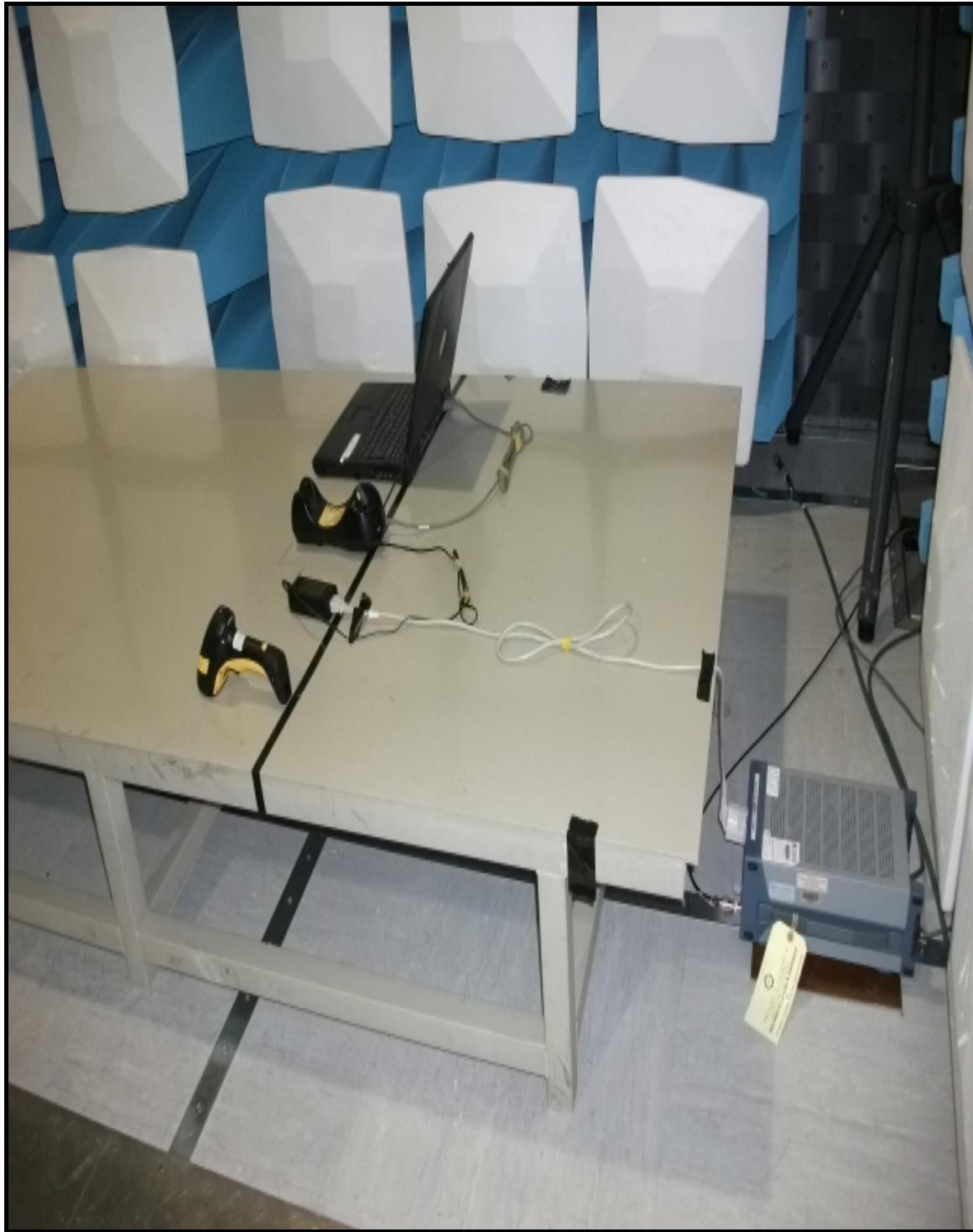
**PHT\77263JD03\003 - Test Configuration Photograph - Radiated Emissions (In cradle)**
