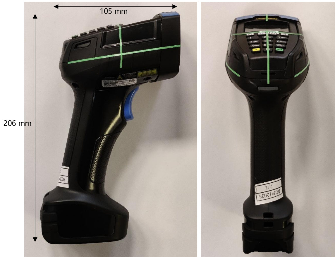
Figure 1 Overview of the DUT
