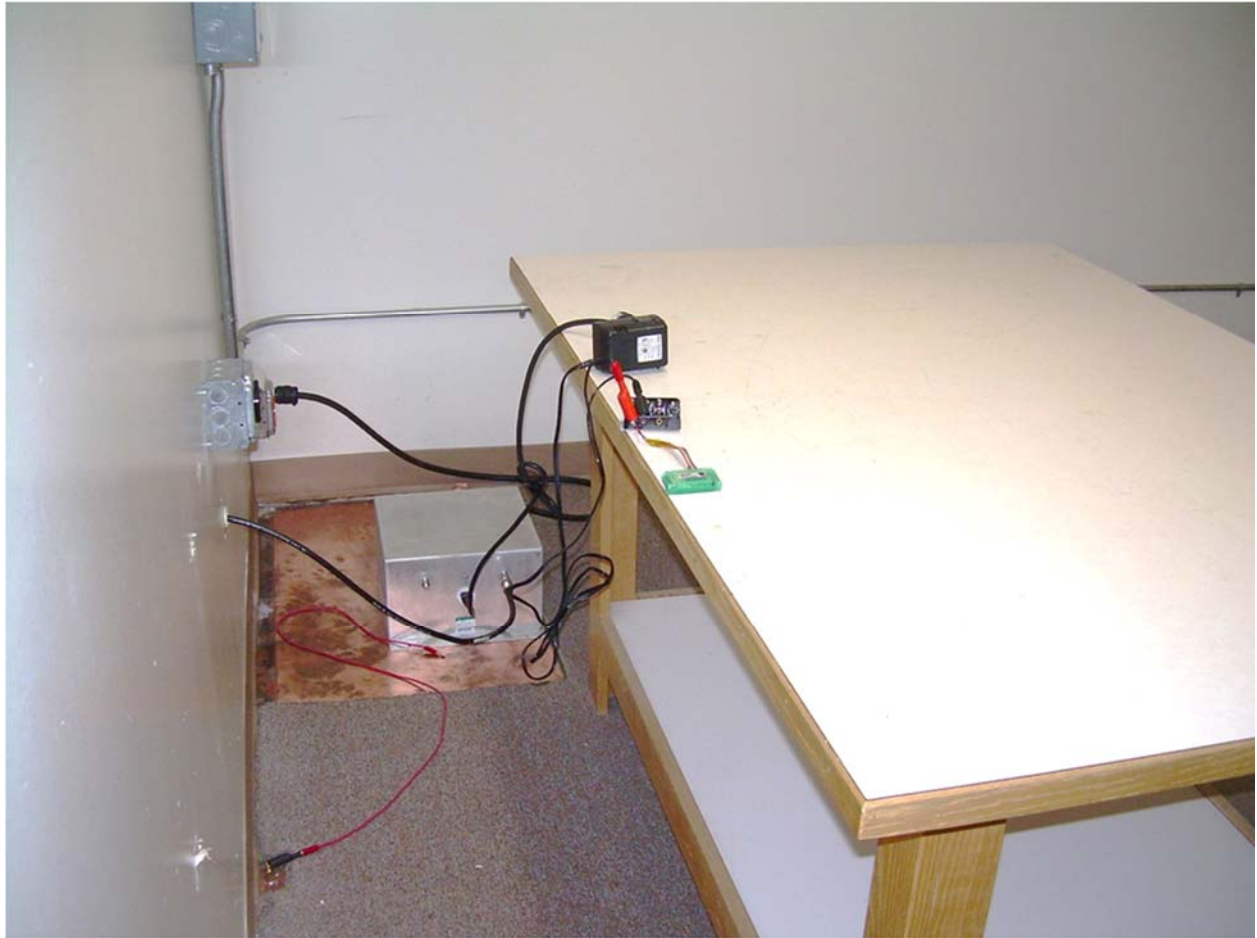
Back View Conducted Disturbance Worst Case Configuration
