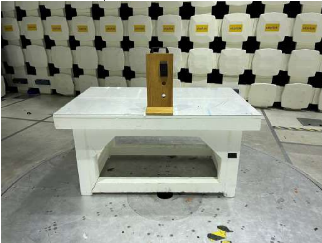
Test Setup With Metal Enclosure, RE 30-1000 MHz
