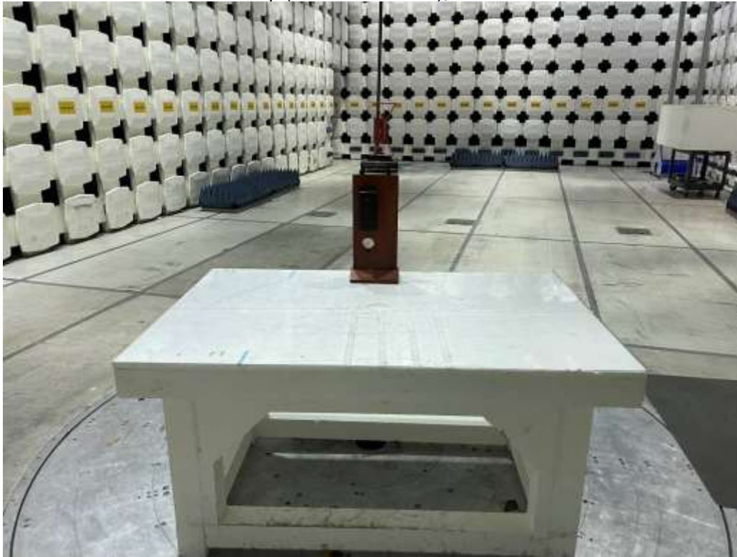
BLE Test Setup (Plastic Enclosure), RE 30-1000 MHz
