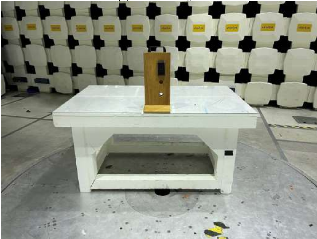
BLE Test Setup (Metal Enclosure), RE 30-1000 MHz
