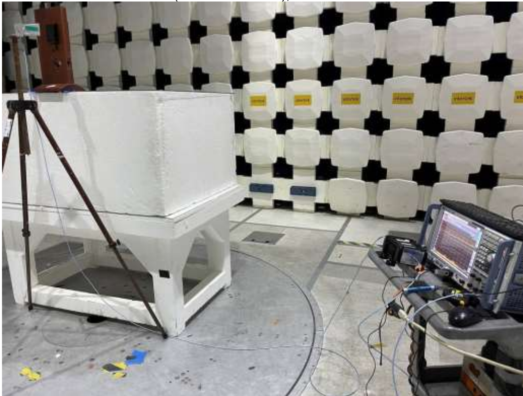
BLE(Plastic Enclosure), RE 18-25 GHz
