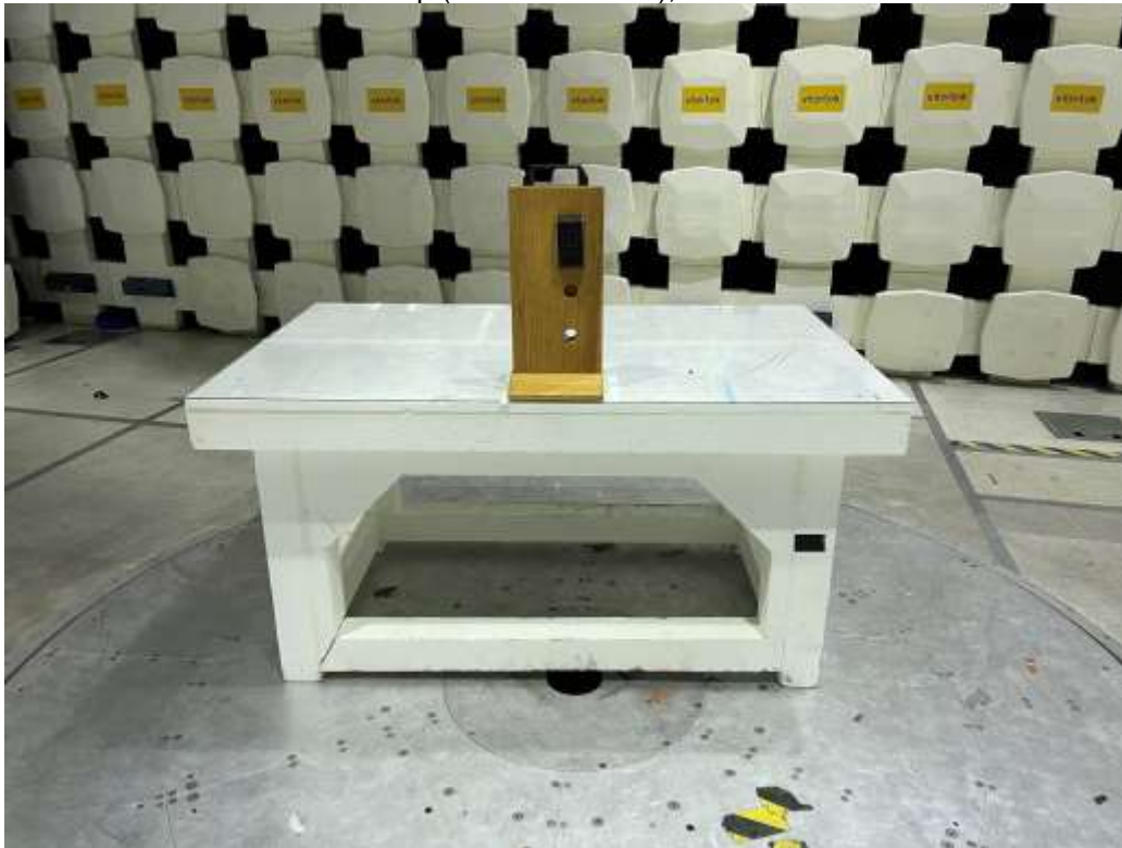
BLE Test Setup (Metal Enclosure), RE 30-1000 MHz
