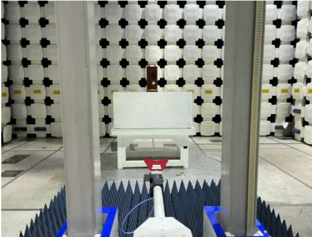
BLE Test Setup (Plastic Enclosure)
