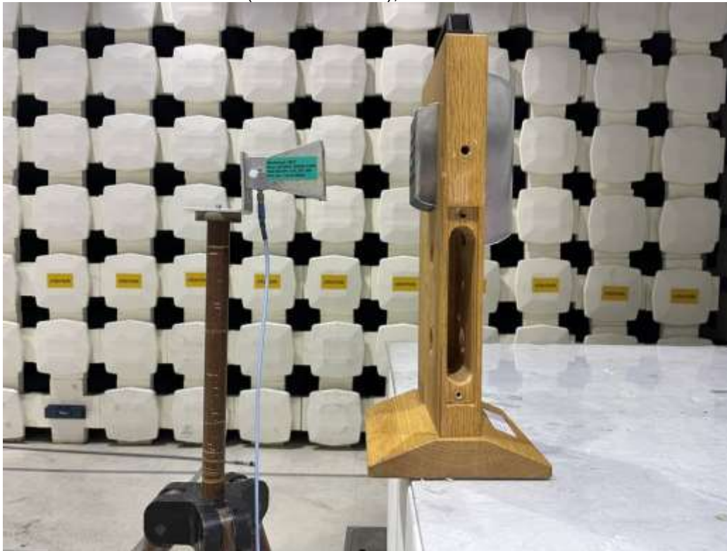
BLE(Metal Enclosure), RE 18-25 GHz
