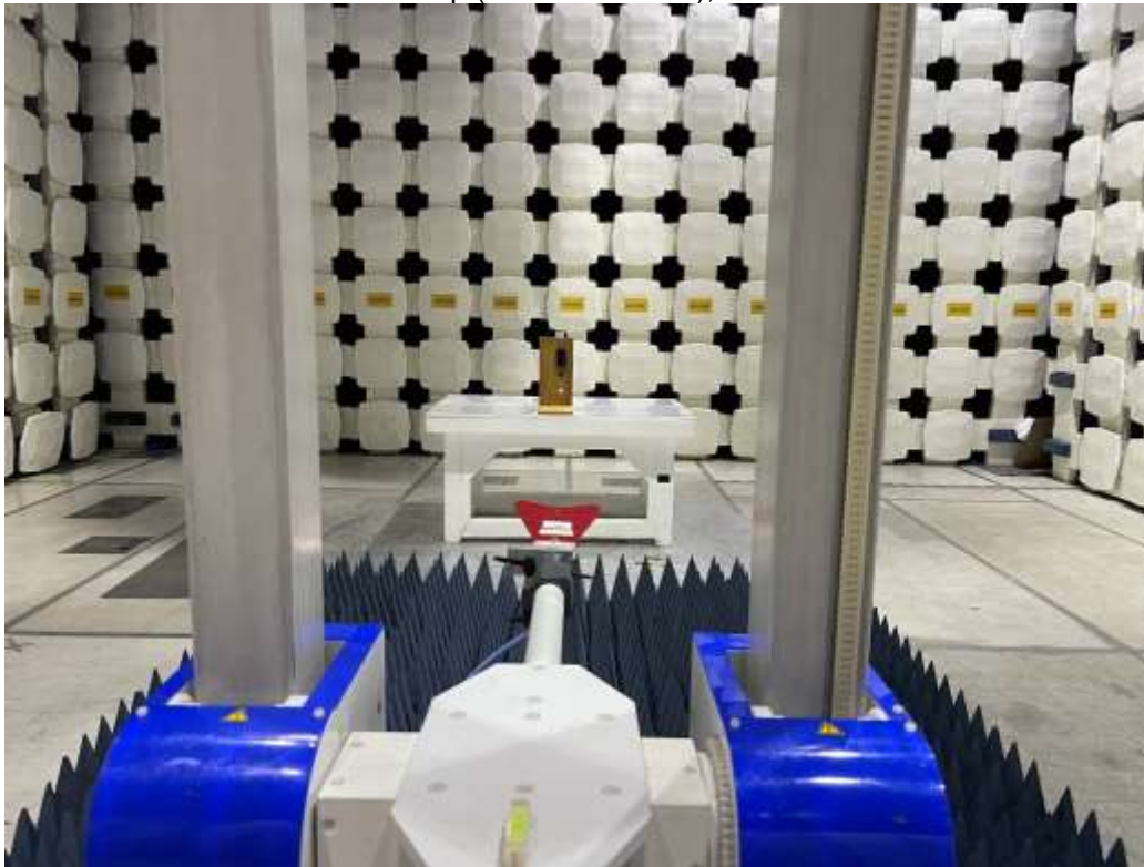
BLE Test Setup (Metal Enclosure), RE 1-13 GHz
