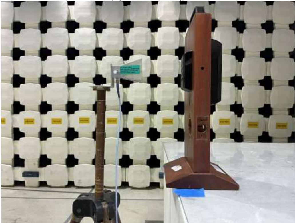
BLE Test Setup (Plastic Enclosure), RE 18-25 GHz
