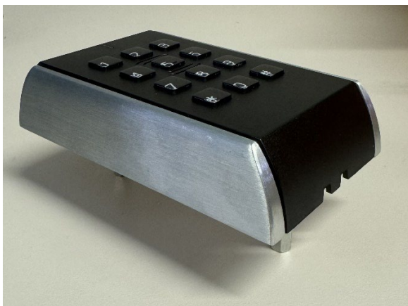
Fig 1: IN100 Keypad Variant plastic cover with metal wings.
