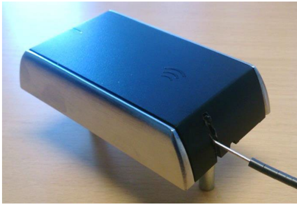
Fig 1: IN100 plastic cover with metal wings.
