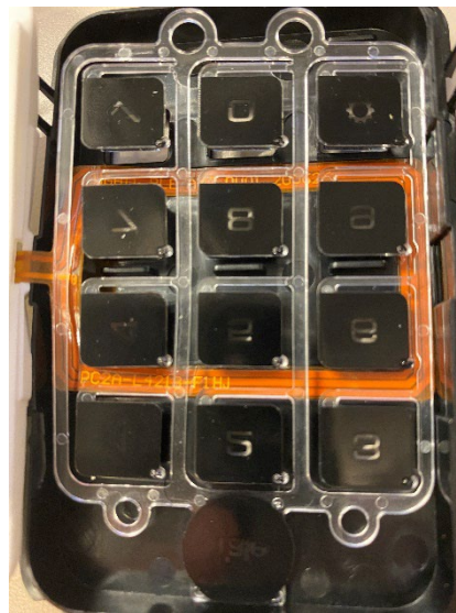
RFID Antenna Behind Push Buttons
