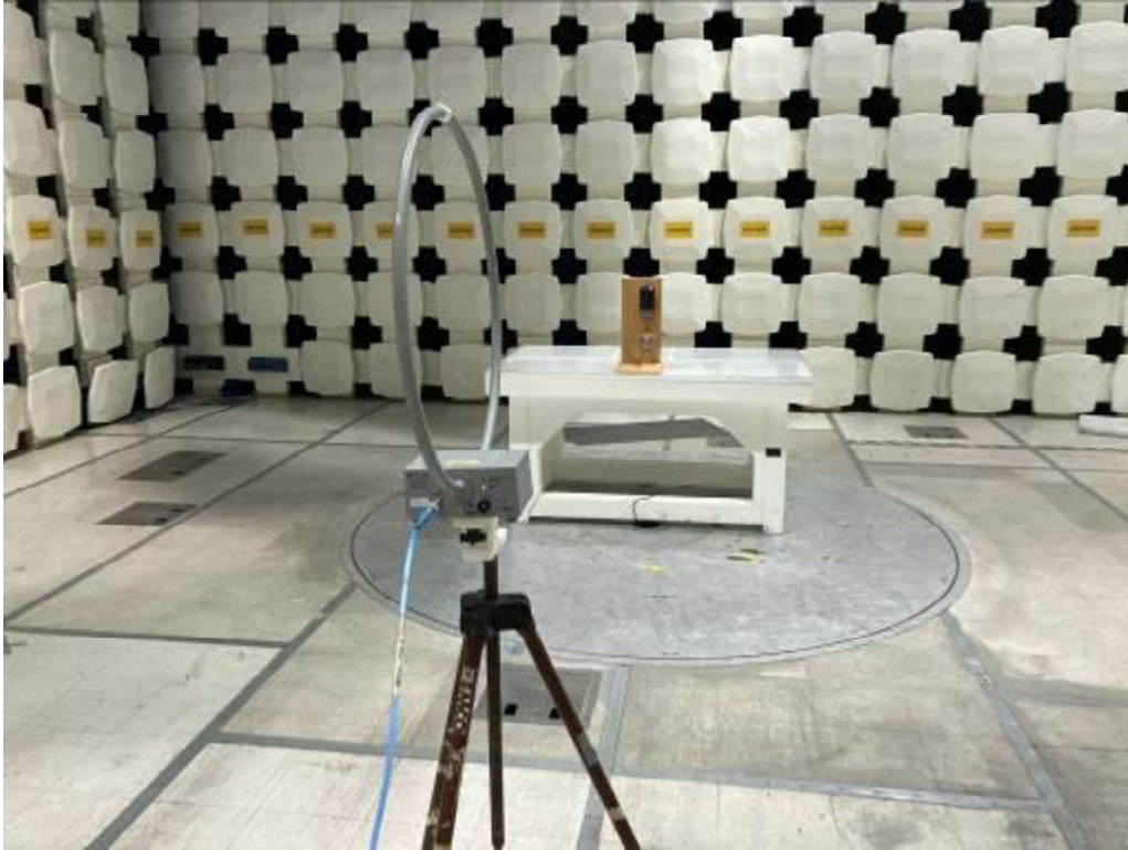
13.56 MHz RFID Test Setup (NTT – Push Button), 9 kHz – 30 MHz, Y-Axis
