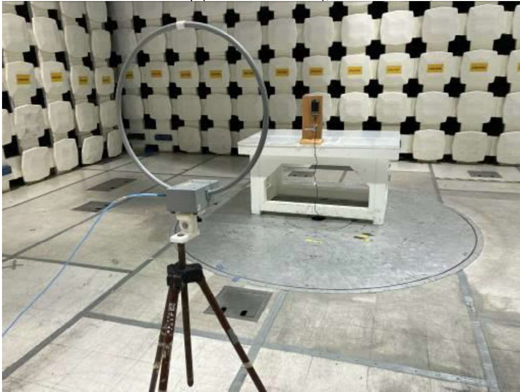
2.4 GHz BLE Test Setup (NTT – Push Button), 9 kHz – 30 MHz, X-Axis
