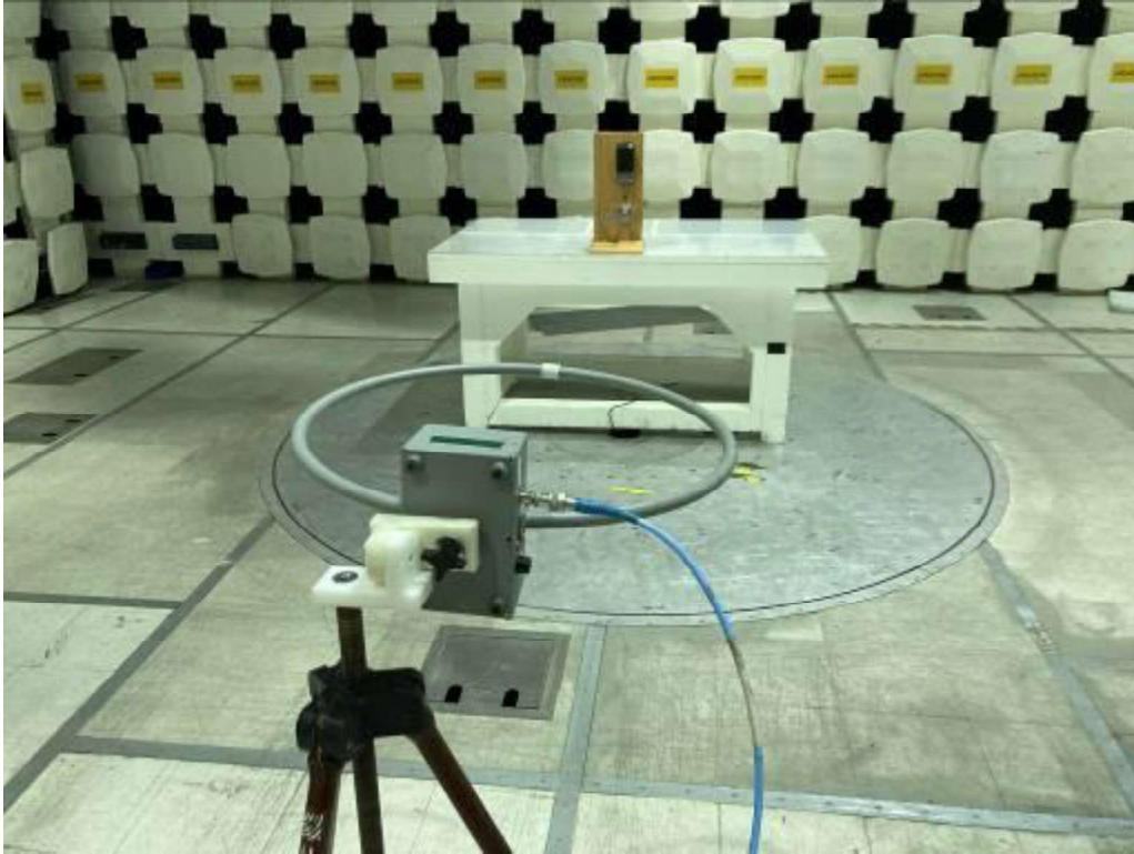
13.56 MHz RFID Test Setup (NTT – Push Button), 9 kHz – 30 MHz, Z-Axis
