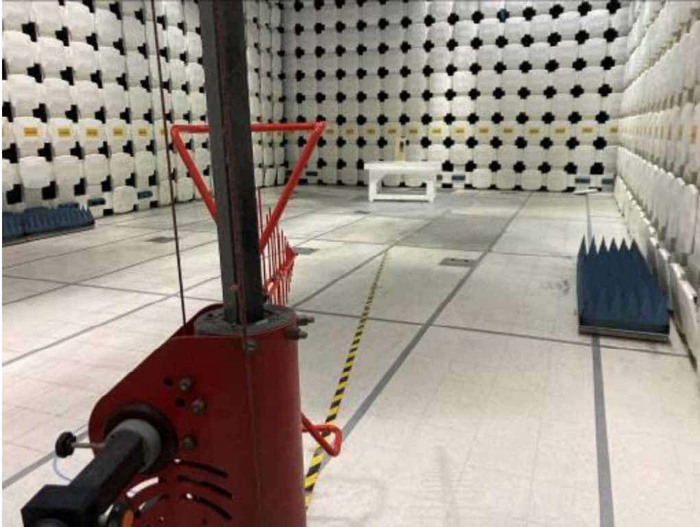
13.56 MHz RFID Test Setup (NTT – Push Button), 30 - 1000 MHz
