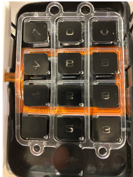
RFID Antenna Behind Push buttons
