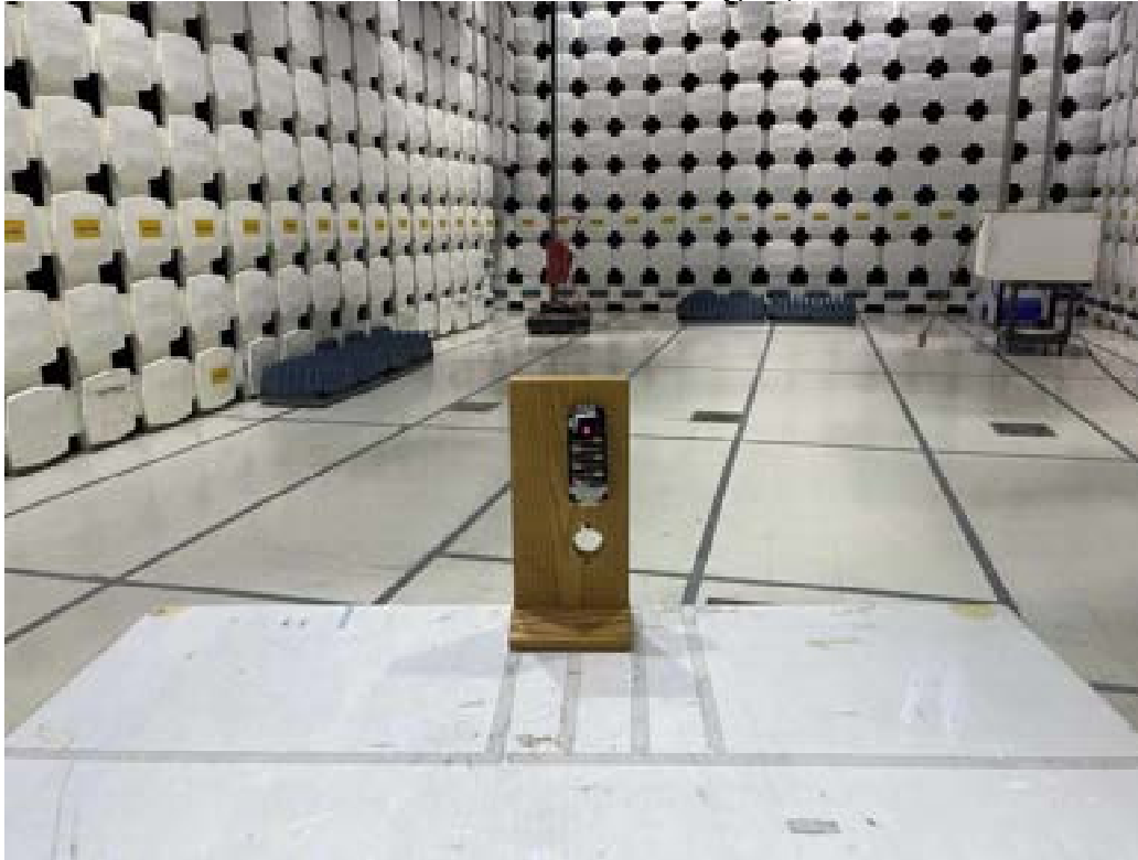
13.56 MHz RFID (Metal Enclosure With Keypad), 30-1000 MHz
