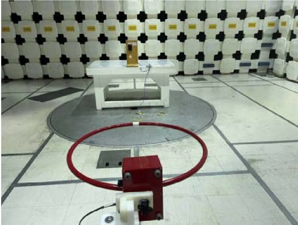
BLE (Plastic Enclosure Without Keypad), 9 kHz – 30 MHz, Antenna on Z-Axis
