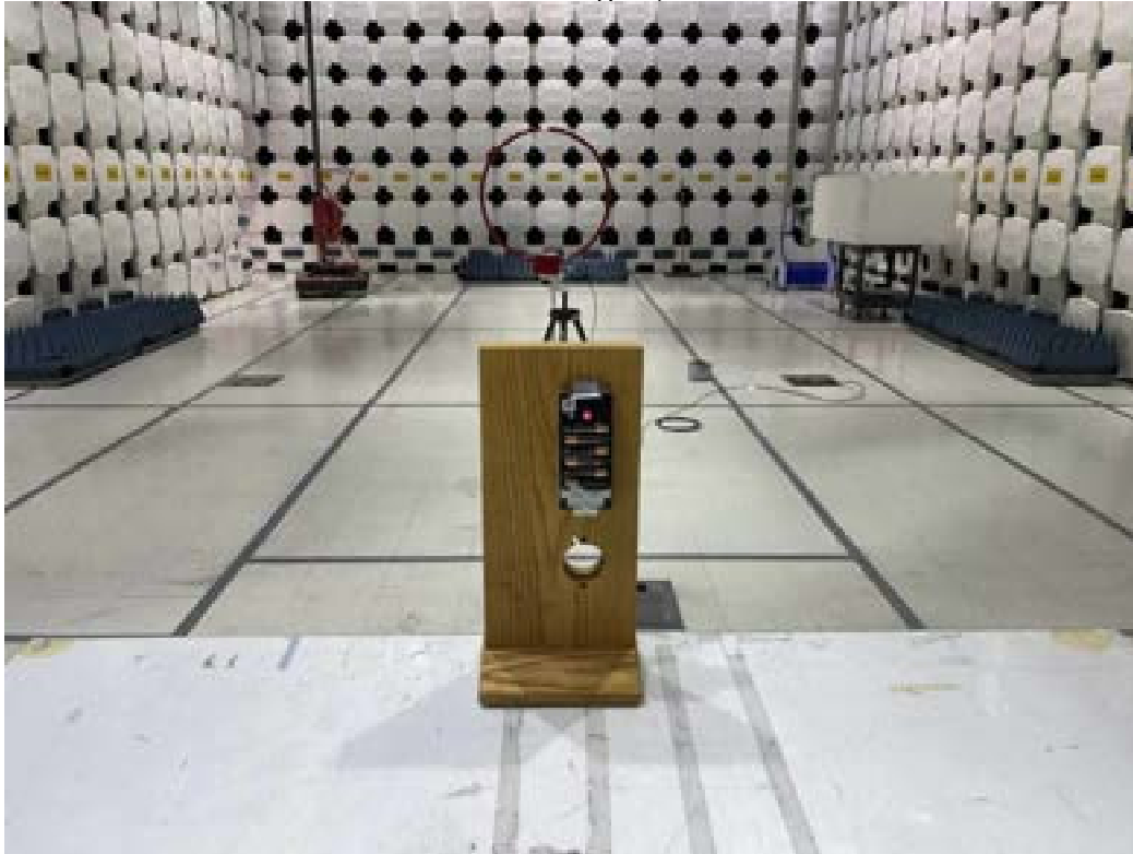
Metal Enclosure Without Keypad, Antenna on X-Axis
