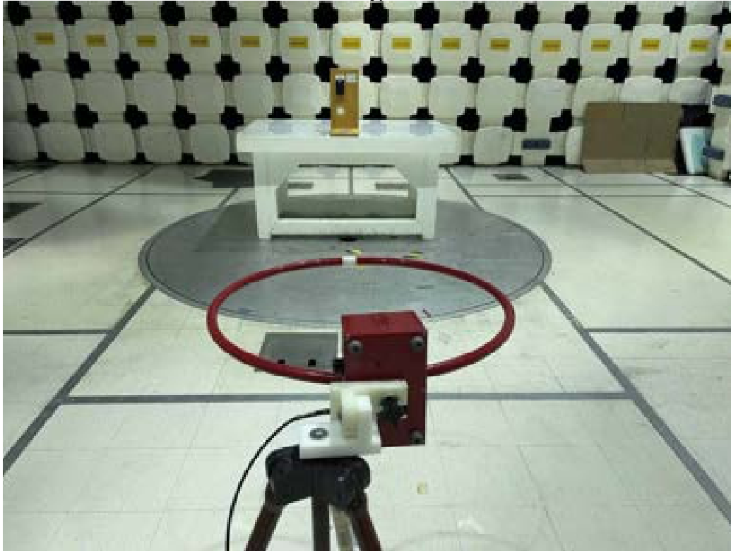
Metal Enclosure With Keypad, Antenna on Z-Axis
