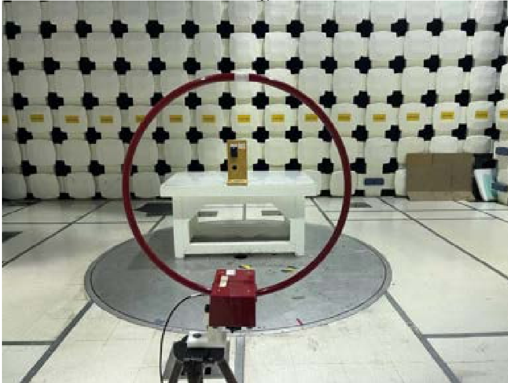
Plastic Enclosure With Keypad, Antenna on X-Axis
