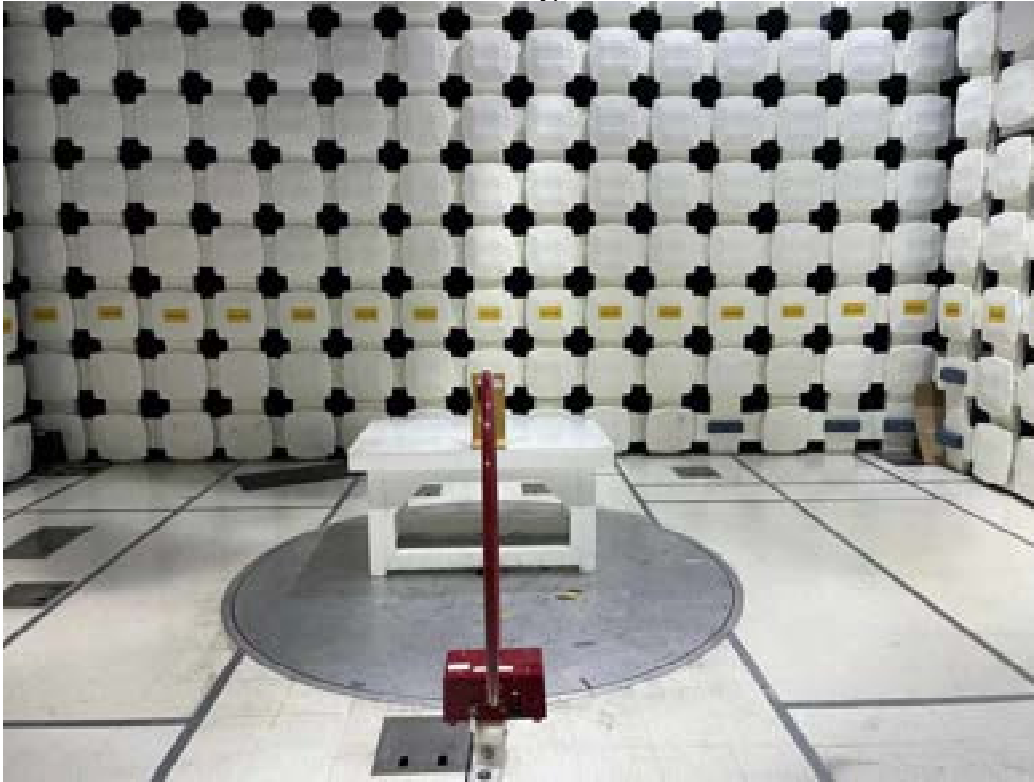
Metal Enclosure Without Keypad, Antenna on Y-Axis
