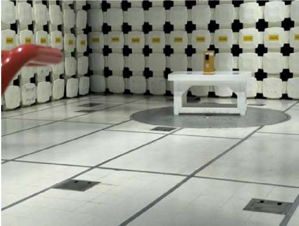
13.56 MHz RFID (Plastic Enclosure Without Keypad), 30-1000 MHz
