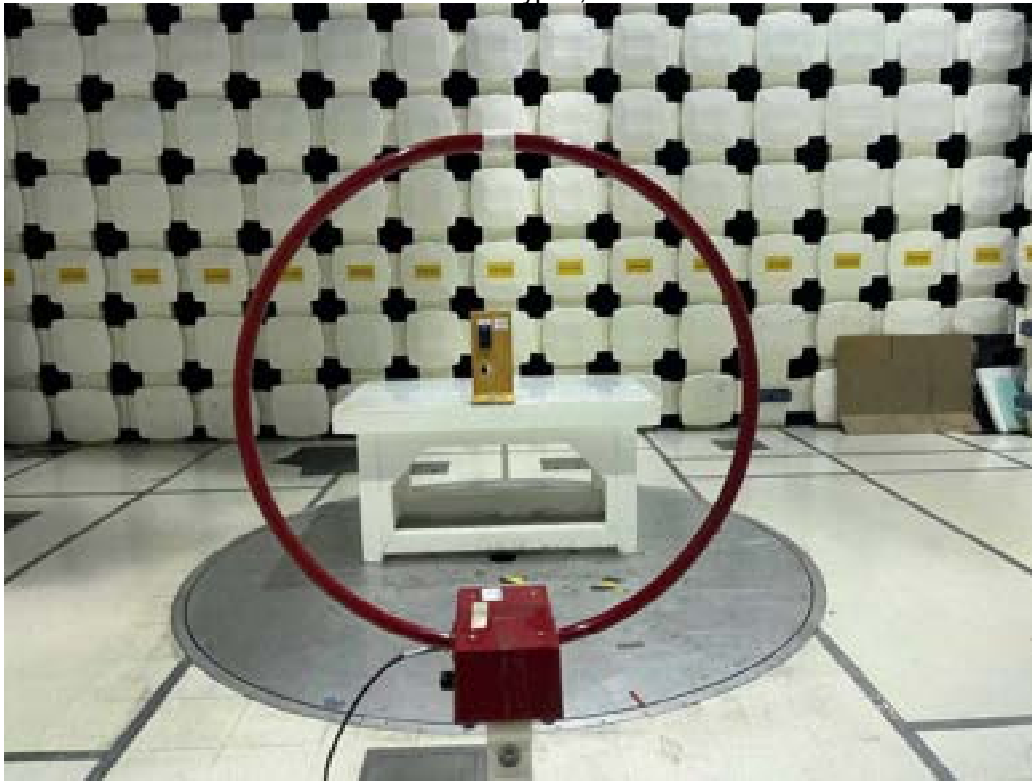
Metal Enclosure With Keypad, Antenna on X-Axis
