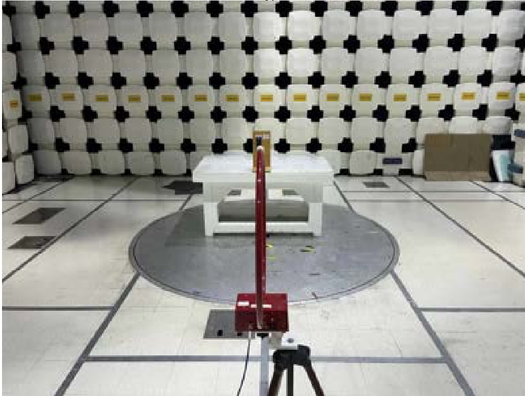
Metal Enclosure With Keypad, Antenna on Y-Axis
