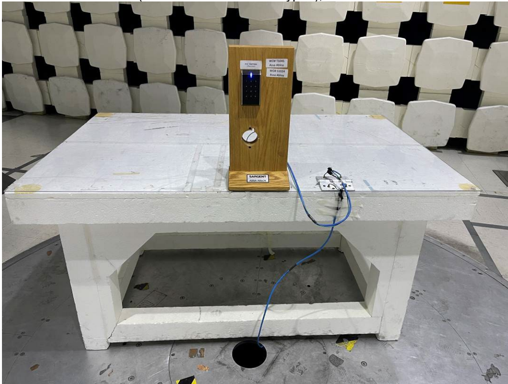
BLE (Metal Enclosure With Keypad), 30-1000 MHz
