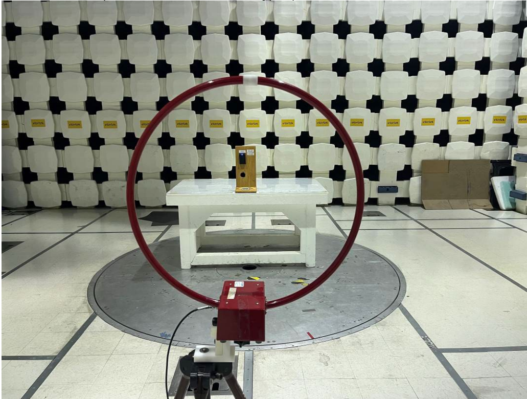
125 kHz RFID (Plastic Enclosure With Keypad), 9 kHz – 30 MHz, Antenna on X-Axis
