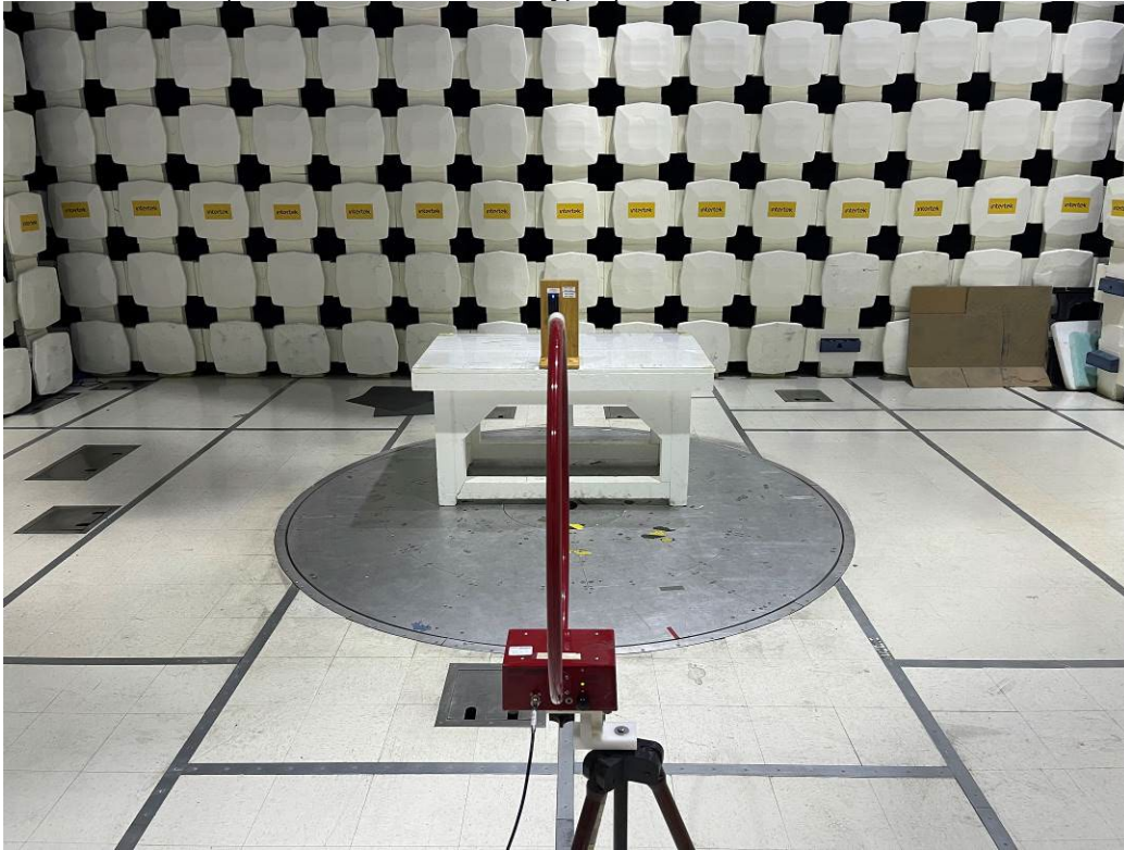
125 kHz RFID (Metal Enclosure With Keypad), 9 kHz – 30 MHz, Antenna on Y-Axis
