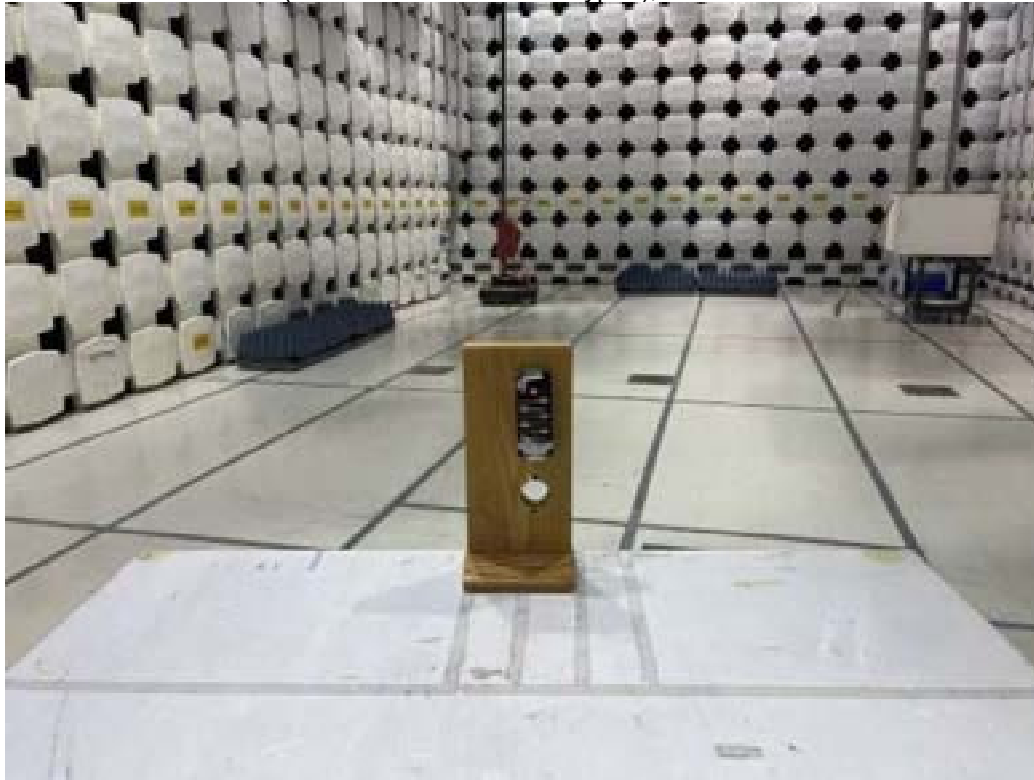
BLE (Metal Enclosure With Keypad), 30-1000 MHz
