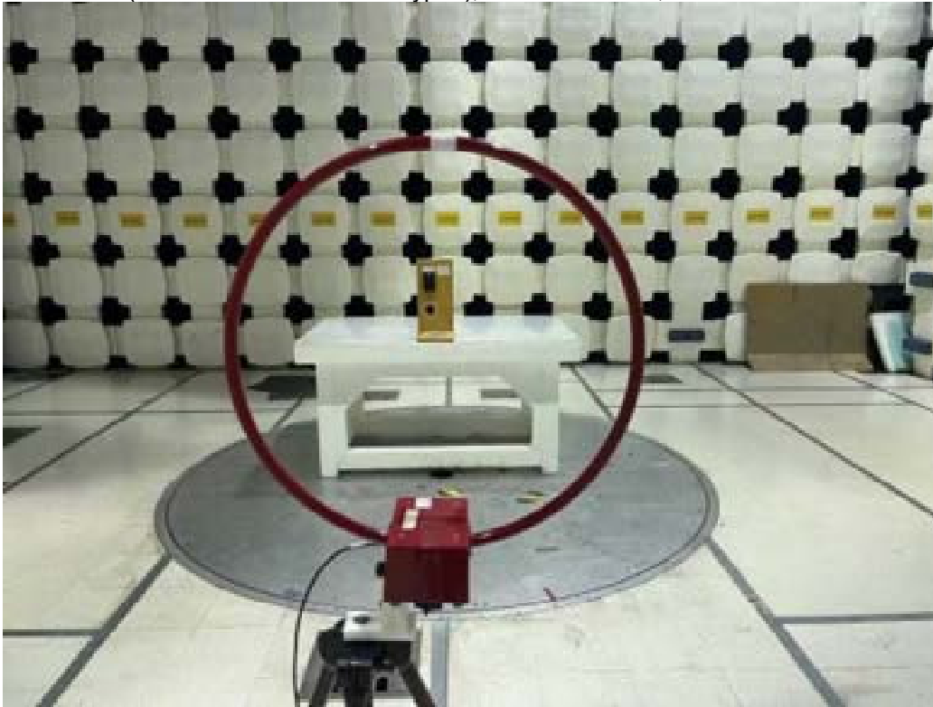
BLE (Plastic Enclosure With Keypad), 9 kHz – 30 MHz, Antenna on X-Axis
