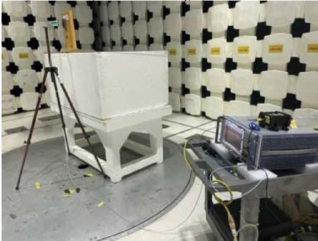
BLE (Metal Enclosure With Keypad), 18-25 GHz
