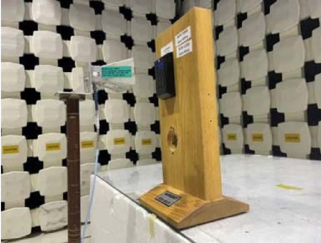
BLE (Plastic Enclosure With Keypad), 18-25 GHz
