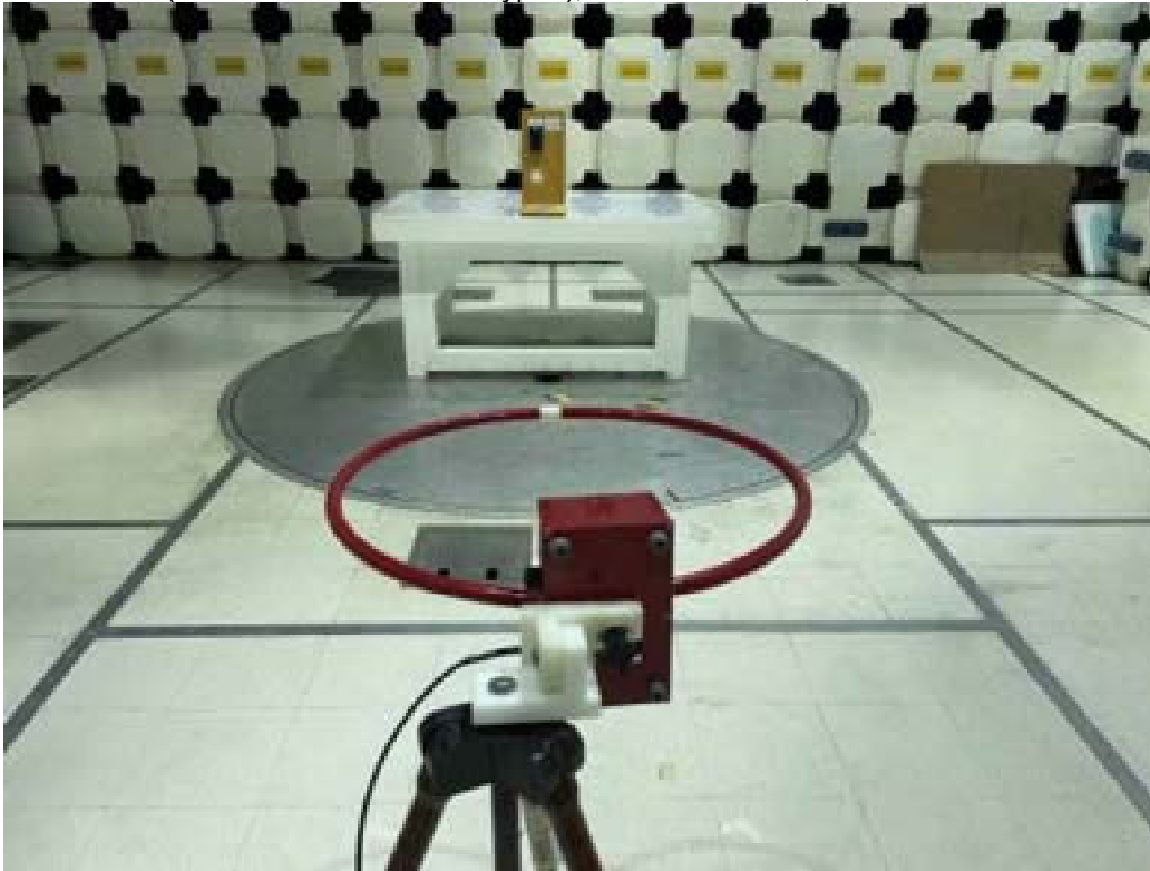
BLE (Metal Enclosure With Keypad), 9 kHz – 30 MHz, Antenna on Z-Axis
