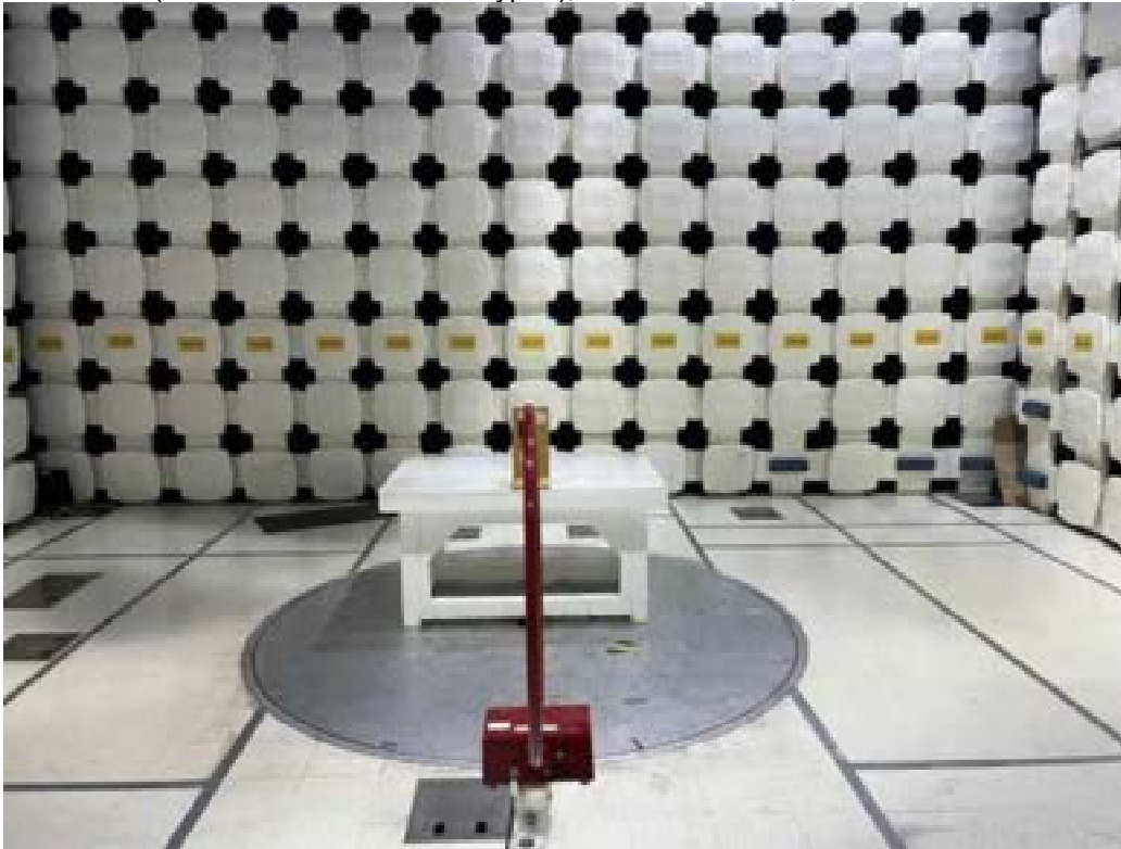
BLE (Plastic Enclosure With Keypad), 9 kHz – 30 MHz, Antenna on Y-Axis
