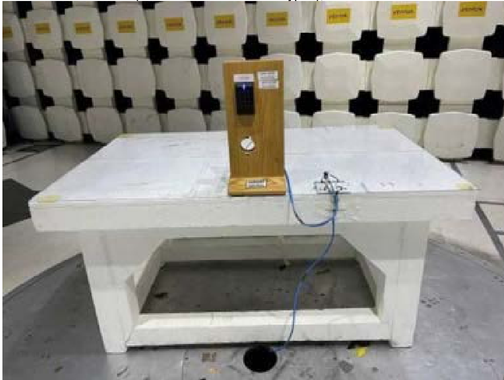
BLE (Plastic Enclosure With Keypad), 30-1000 MHz
