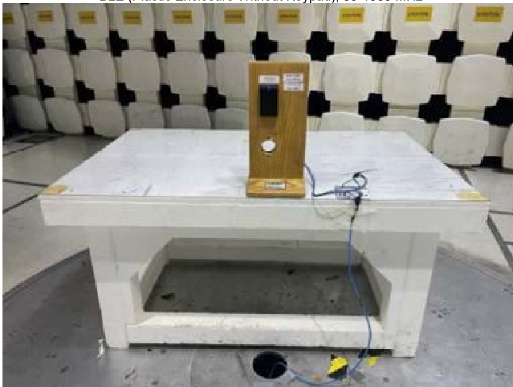
BLE (Plastic Enclosure Without Keypad), 30-1000 MHz
