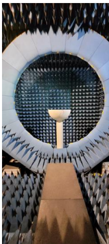
Figure 5-18 Satimo SG-23 6 GHz Stargate Antenna Test Chamber.
