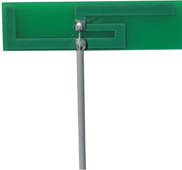
Figure 5-1 UHF antenna element used in Assa Sargent Aurora
