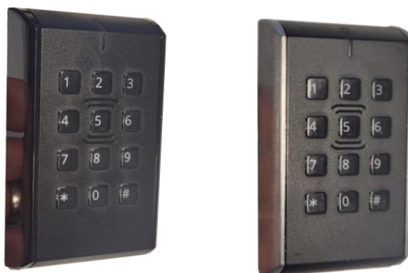
Figure 5-3 Aurora door lock front covers; left plastic cover, right plastic cover with metal wings.
