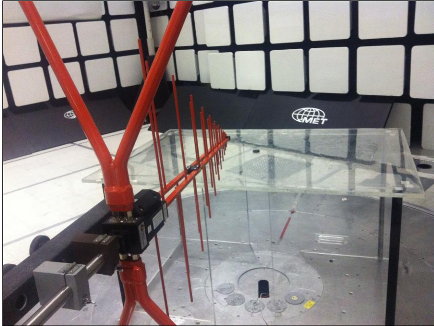
Photograph 3. Radiated Spurious Emissions, Test Setup, 30 MHz – 1 GHz
