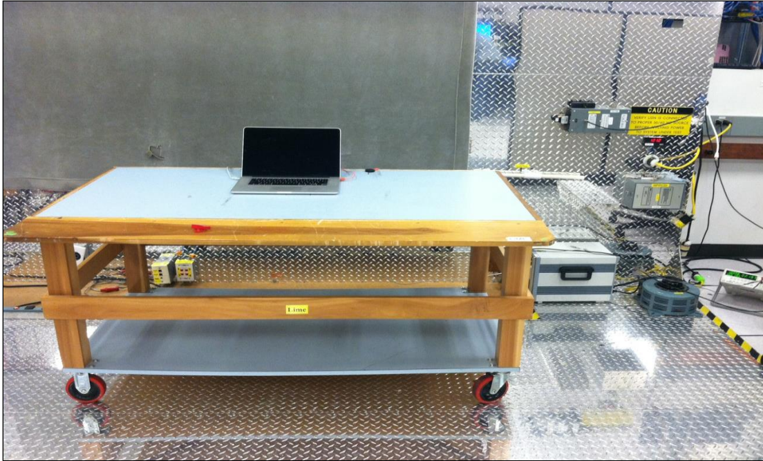
Photograph 1. Conducted Emissions, 15.207(a), Test Setup
