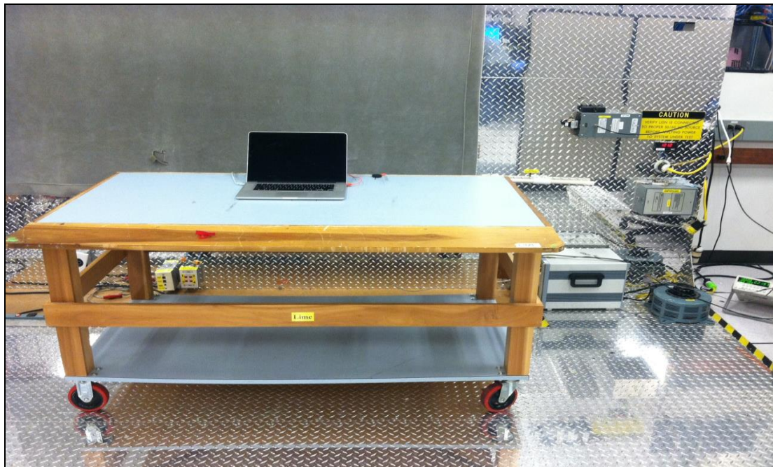
Photograph 2. Conducted Emissions, 15.207(a), Test Setup
