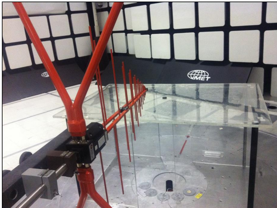
Photograph 4. Radiated Spurious Emissions, Test Setup, 30 MHz – 1 GHz
