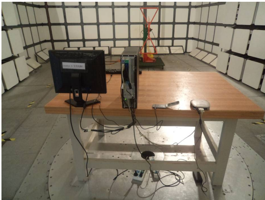
Radiated Emissions - Rear View (30 MHz-1GHz)
