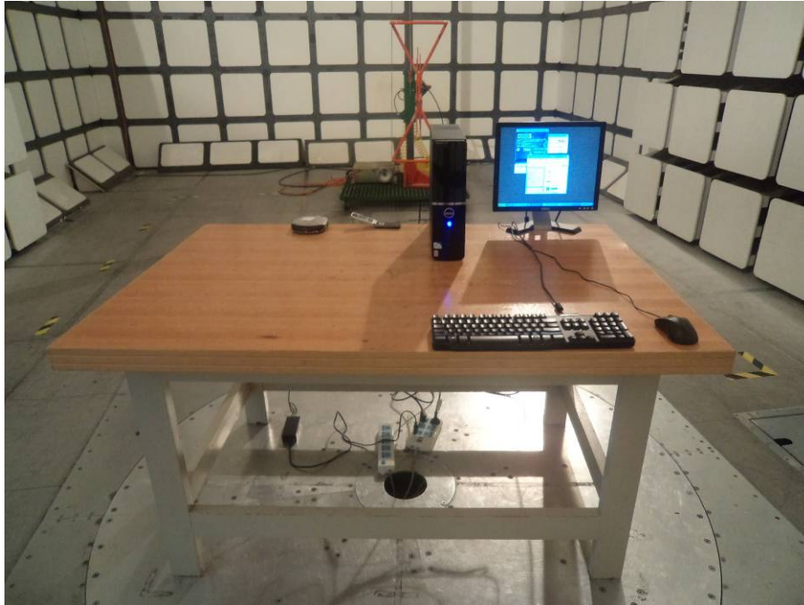
Radiated Emissions - Front View (30 MHz-1GHz)
