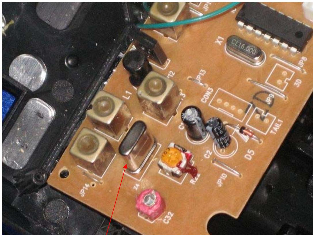
The Crystal is soldered on the PCB
