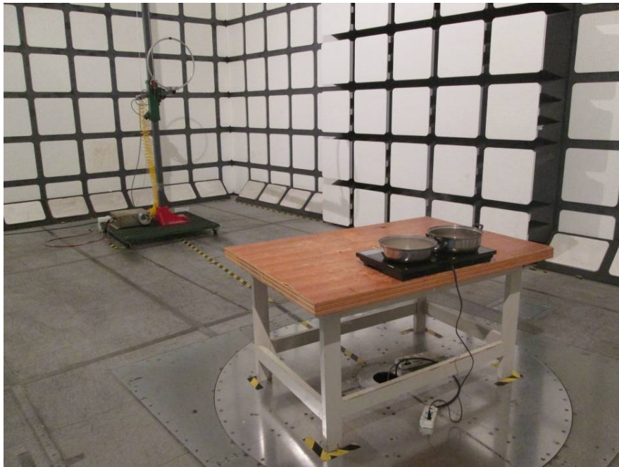
Radiated Emissions - Rear View
