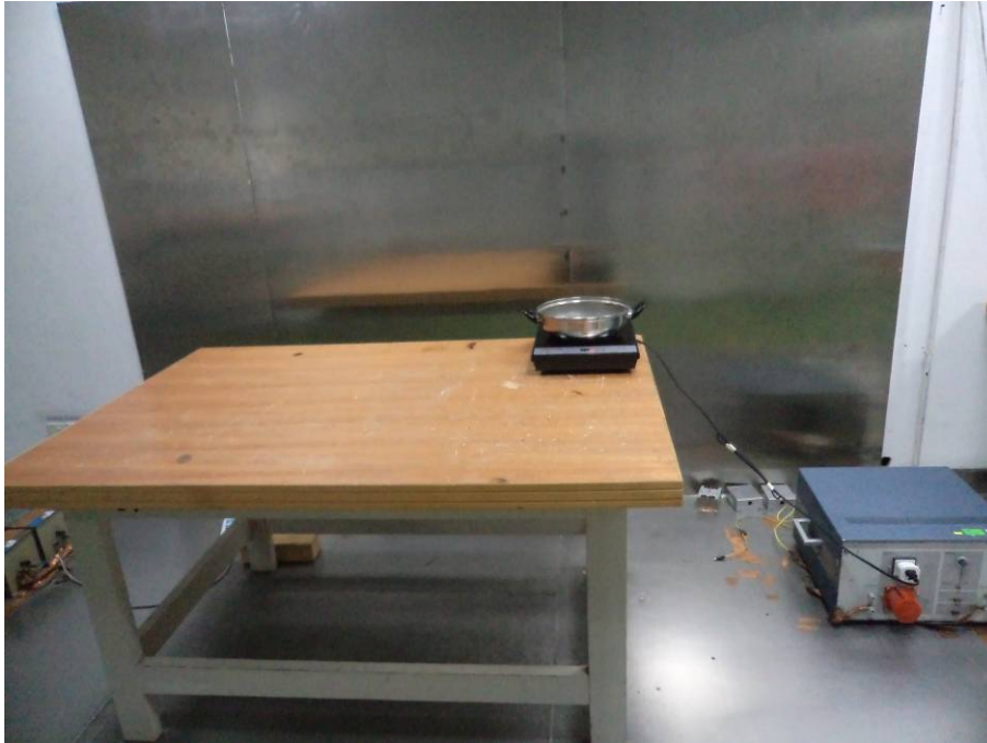
AC Line Conducted Emissions – Side View
