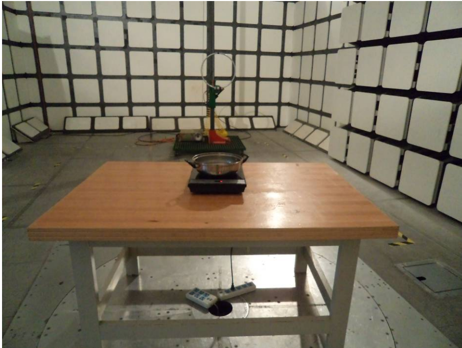
Radiated Emissions – Front View
