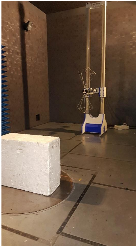
Radiated measurement setup between 200 MHz to 1000 MHz
