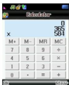
Using this feature, you can use the phone as a calculator. The calculator performs the basic arithmetic functions and memory functions; Addition, Subtraction, Multiplication and Division; Add to Memory, Subtract to Memory, Memory Clear and Memory Read.
