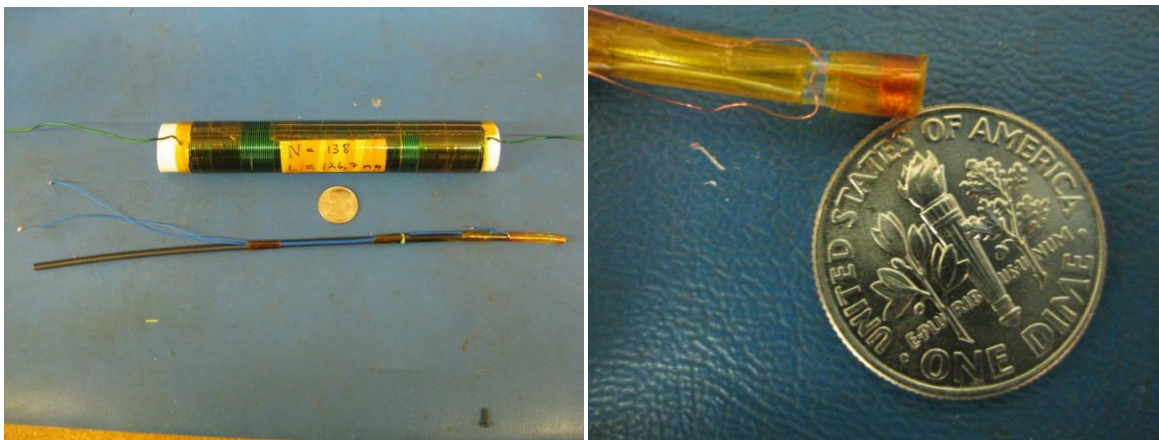
Figure 3 Sensor and Calibration Windings
