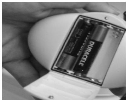
Insert 3 AAA batteries. Close the lid and screw tightly shut to ensure a waterproof seal.
