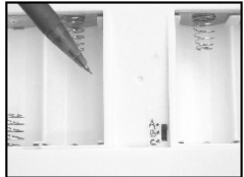
Channels of the Sound Machine and the Sensor must be the same or the unit will not function in auto mode. Now insert 4 size C batteries, close the lid and place the unit on a flat, dry surface in the bathroom.
