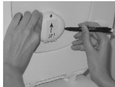
1. Raise the SEAT and the LID of your toilet. (The TT sensor should be installed on the lid with both the seat and lid up to be sure it will not hit the seat when they are both down)
