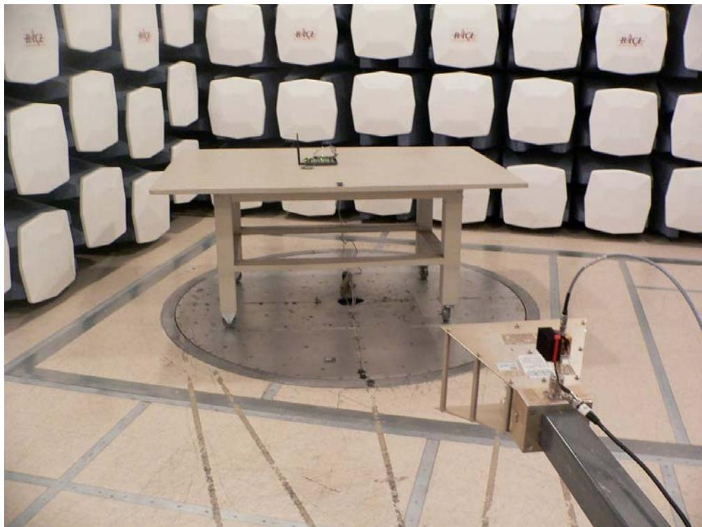
**10.6 Transmitter Radiated Spurious Emissions – Rear View**
