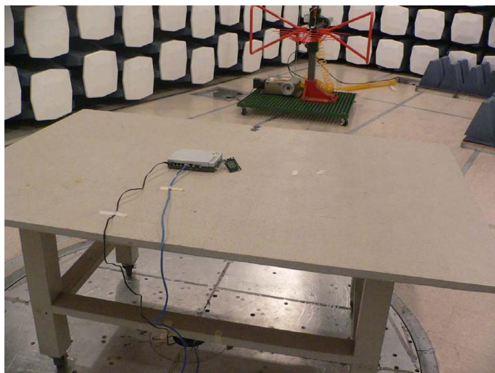
**10.5 Transmitter Radiated Spurious Emissions – Front View**
