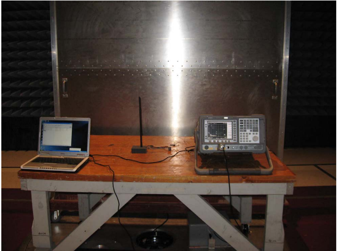
Photograph 2. Conducted Emissions Test Setup
