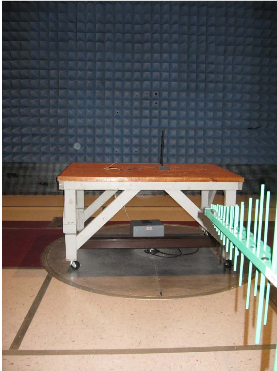
Photograph 3. Radiated Emission Test Setup 30 MHz - 1 GHz
