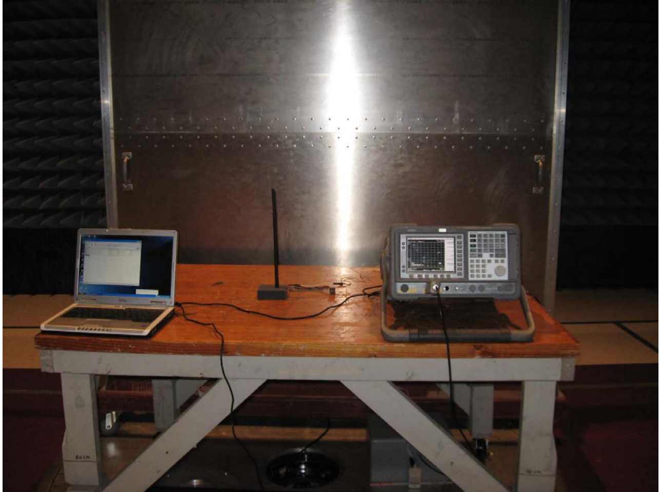
Photograph 4. Conducted Emissions Test Setup
