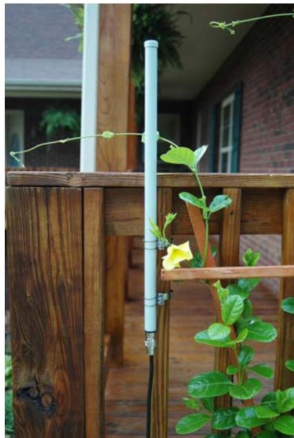
Install the antenna with the hardware included. The antenna should be mounted vertically.
