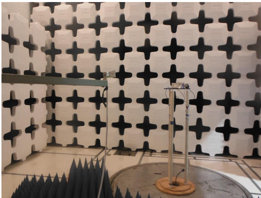
Figure 2: Radiated Emission 18GHz-25GHz set up
