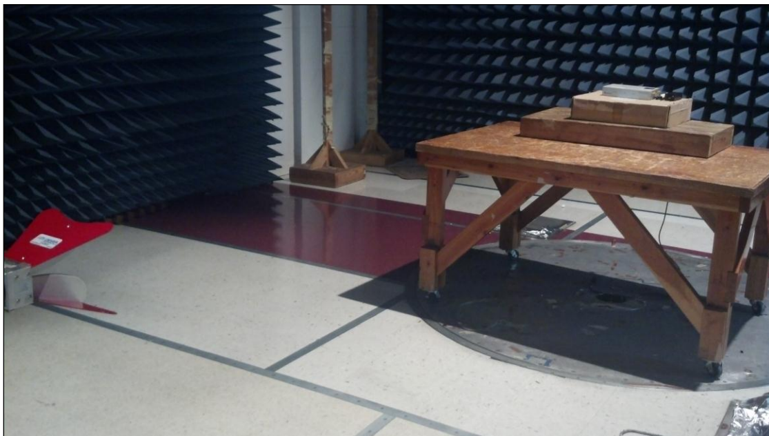
Photograph 2. Radiated Spurious Emissions, Test Setup, Above 1 GHz
