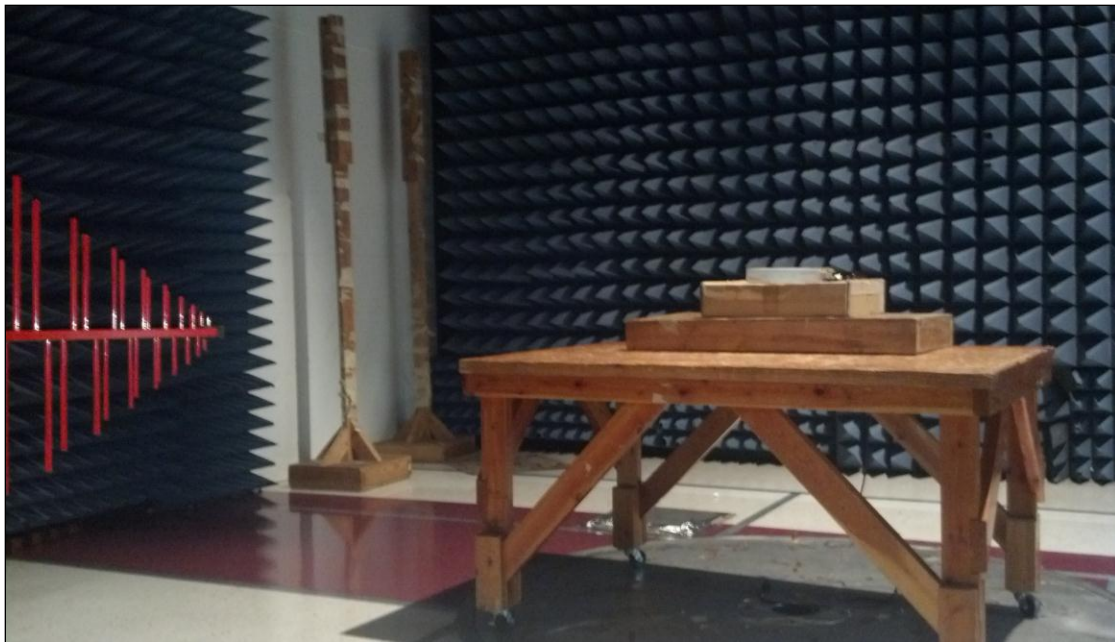
Photograph 1. Radiated Spurious Emissions, Test Setup, 30 MHz – 1 GHz
