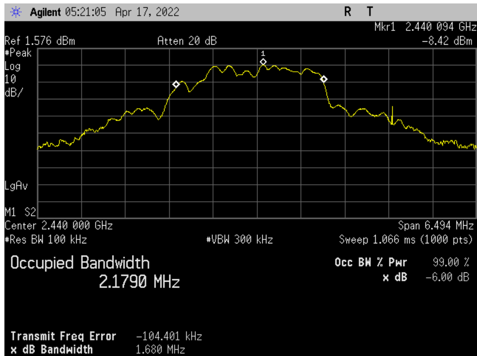
Figure 6. Zigbee_Mid Ch_2440MHz_1MBit_Occupied Bandwidth_-6dB_Port 1.
