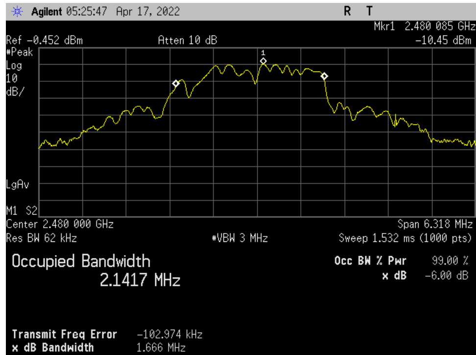
Figure 9. Zigbee_High Ch_2480MHz_1MBit_Occupied Bandwidth_99 percent_Port 1.
