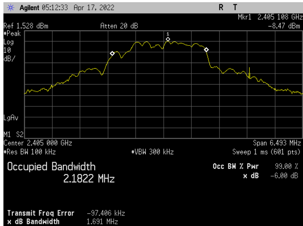
Figure 4. Zigbee_Low Ch_2405MHz_1MBit_Occupied Bandwidth_-6dB_Port 1.
