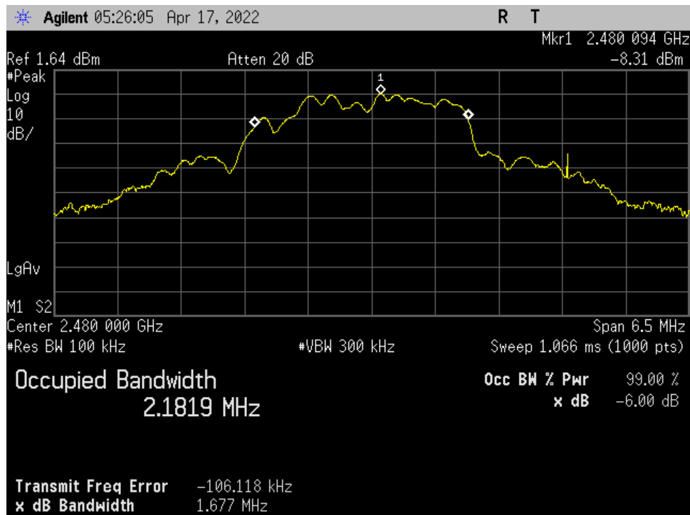
Figure 8. Zigbee_High Ch_2480MHz_1MBit_Occupied Bandwidth_-6dB_Port 1.
