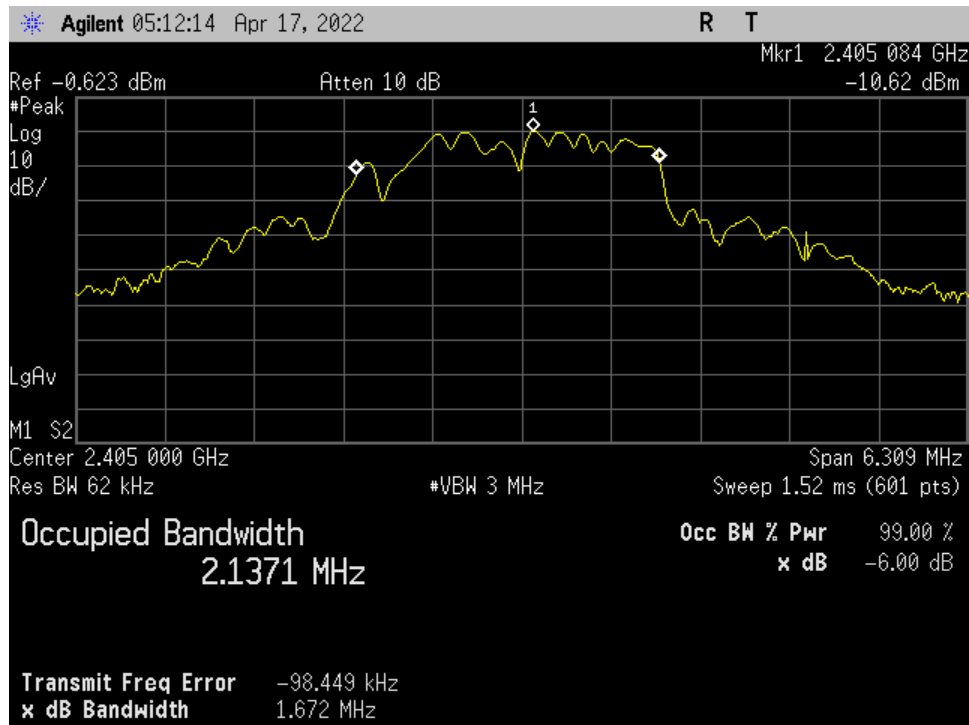
Figure 5. Zigbee_Low Ch_2405MHz_1MBit_Occupied Bandwidth_99 percent_Port 1.
