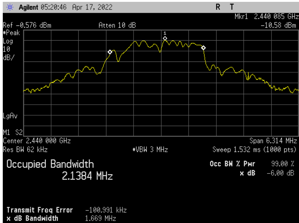
Figure 7. Zigbee_Mid Ch_2440MHz_1MBit_Occupied Bandwidth_99 percent_Port 1.
