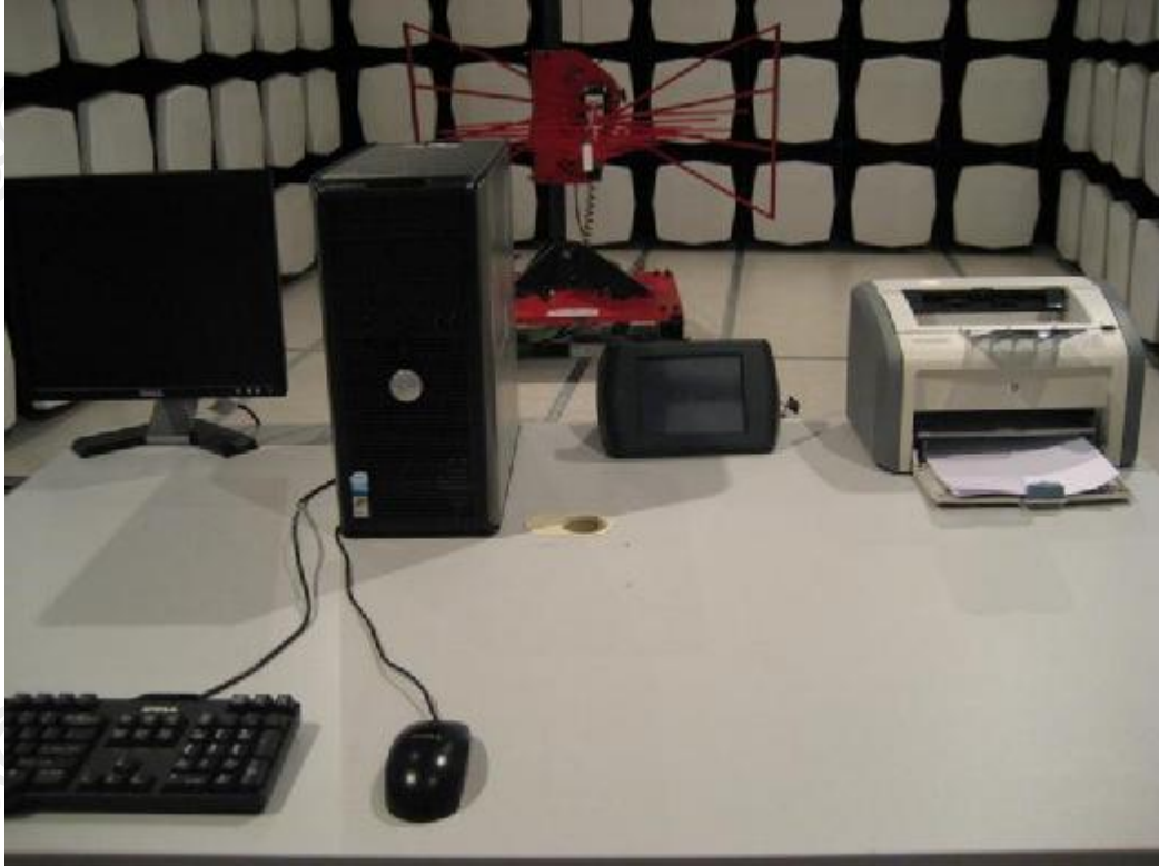
Measurement of Radiated Emission Test Set Up
