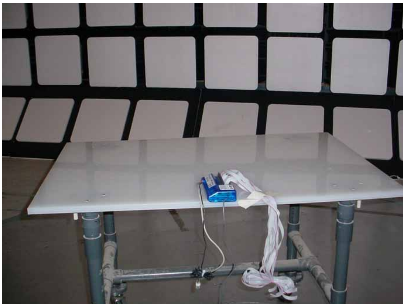
Radiated Emission at 3 m Distance
