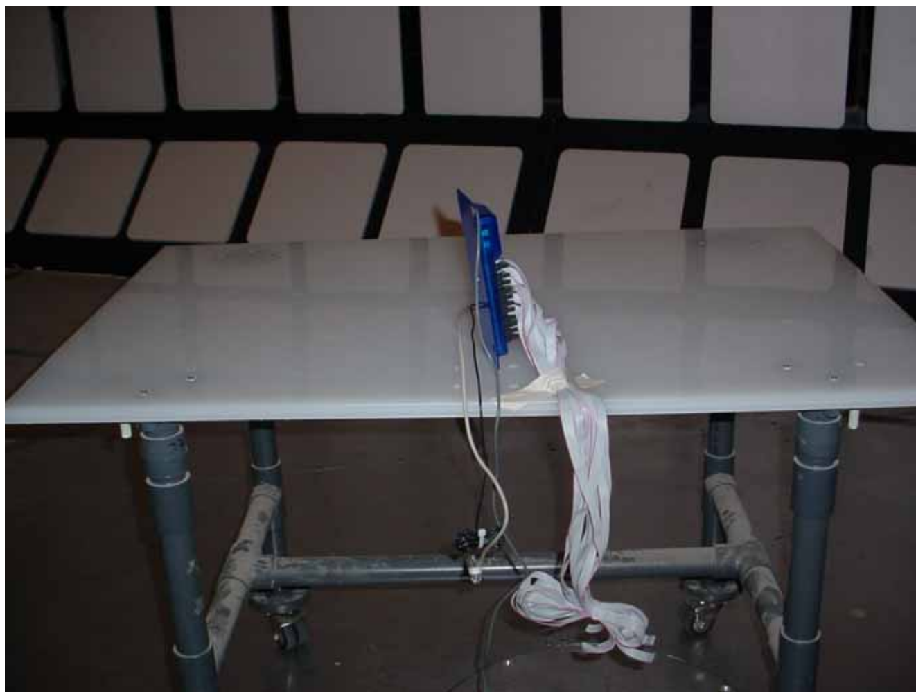
Radiated Emission at 3 m Distance
