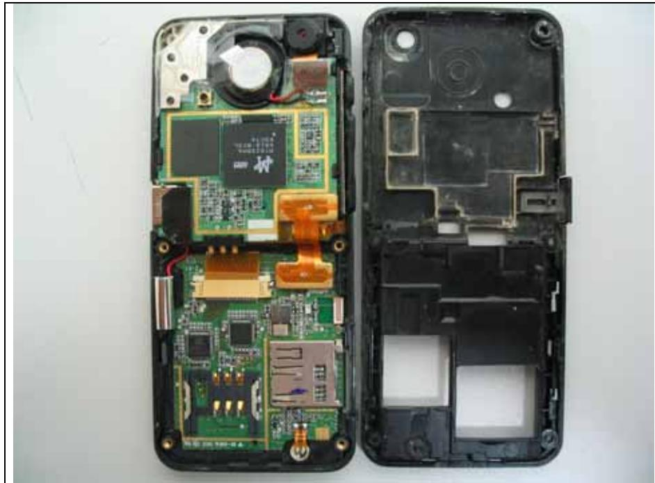
**Top View of Main-board(GSM)**
