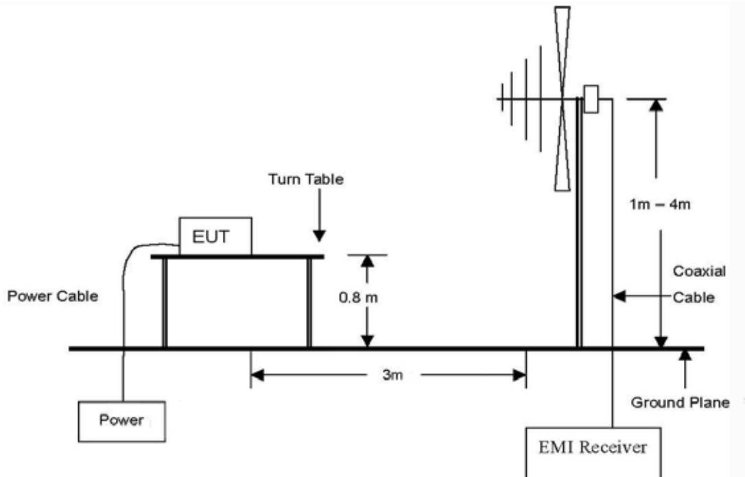
The diagram below shows the test setup that is utilized to make the measurements for emission from 1 GHz to 18 GHz Emissions.
