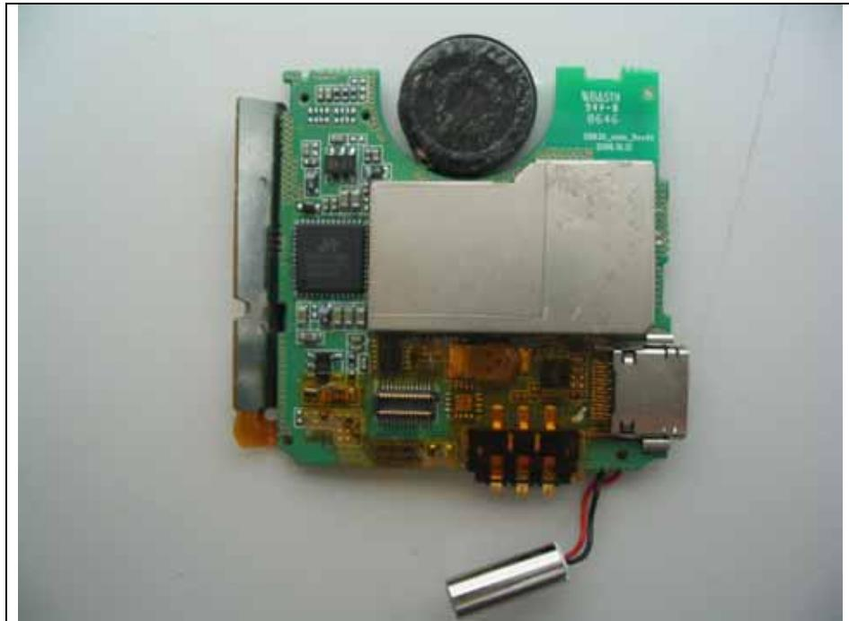
**Bottom View of Main-board(GSM)-Removed shield cap**
