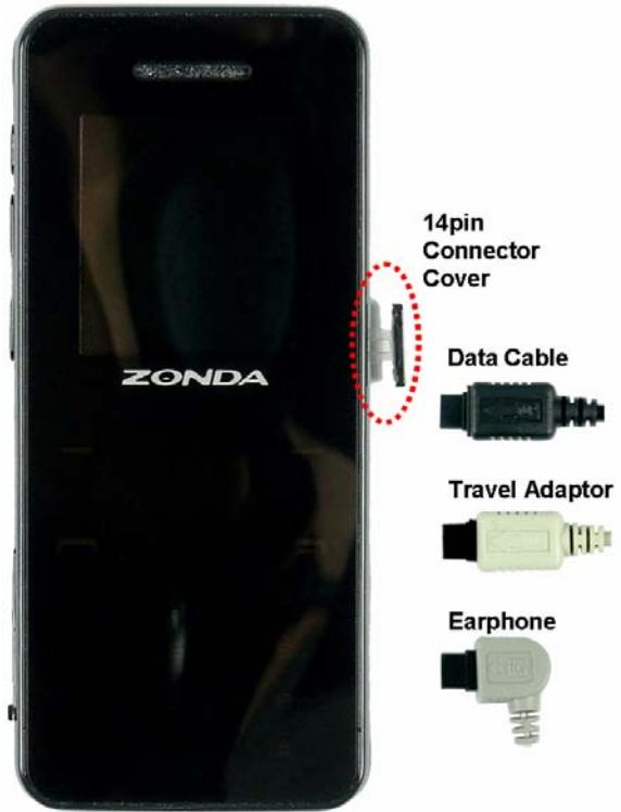
**! Note :** 14pin connector has a direction. Check whether the front side of the jacks of data cable, travel adaptor and earphone marked as 'right arrow' or 'top'. (In case of Data cable and Earphone, use inverse direction)
