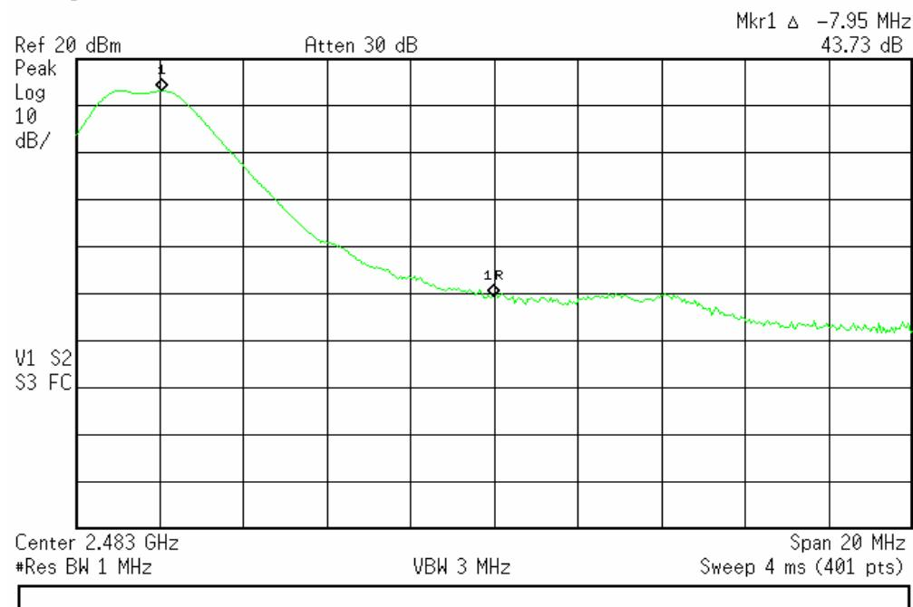
**Conclusion:** The emission at the bandedge is >20dB below the level of the fundamental
