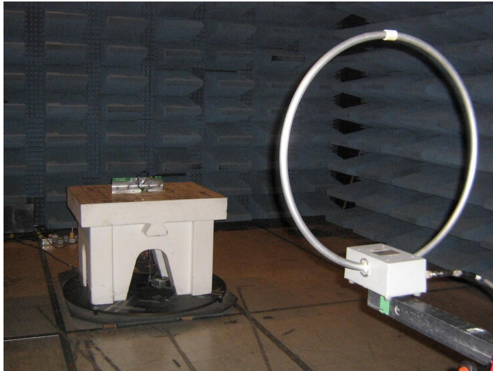
Figure 2: Radiated Emissions (below 30 MHz) Test Setup
