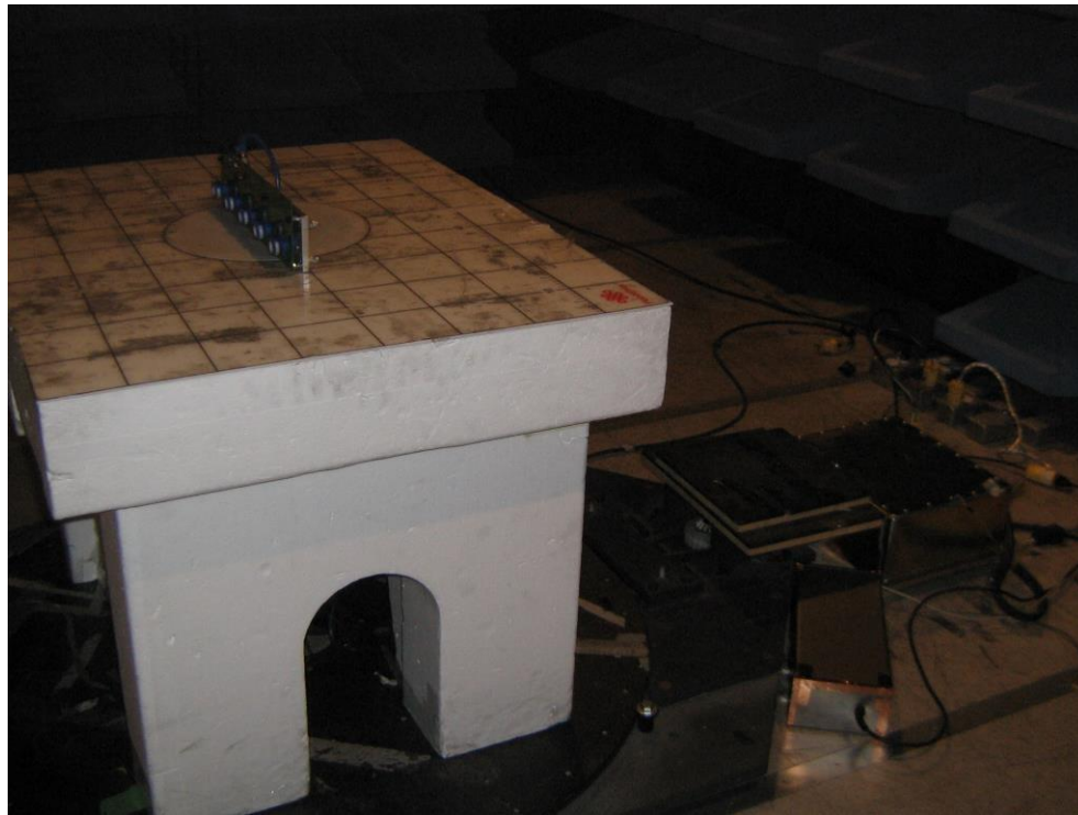
Figure 3: Radiated Emissions Test Setup
