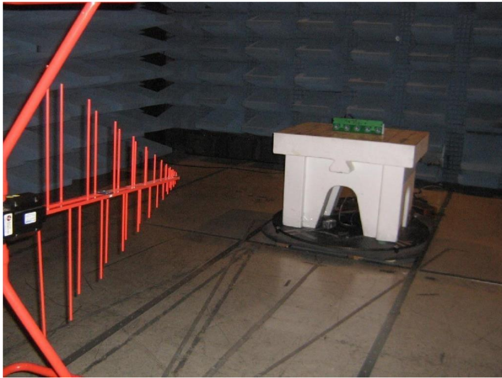
Figure 1: Radiated Emissions (30 MHz – 1 GHz) Test Setup
