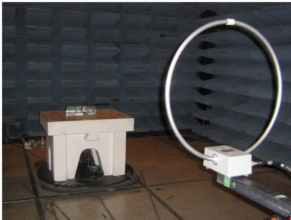
Figure 2: Radiated Emissions (below 30 MHz) Test Setup
