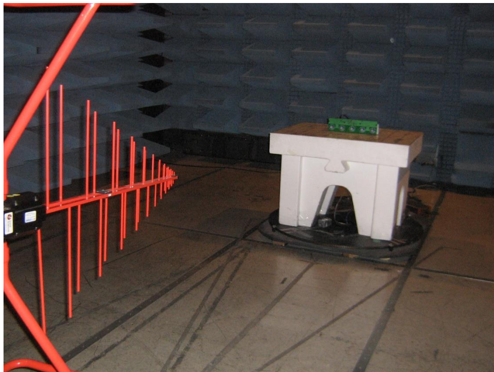
Figure 1: Radiated Emissions (30 MHz – 1 GHz) Test Setup
