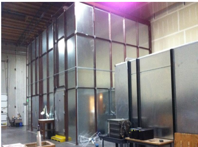
5 m Semi-Anechoic Chamber (SAC) in Everett, Washington
