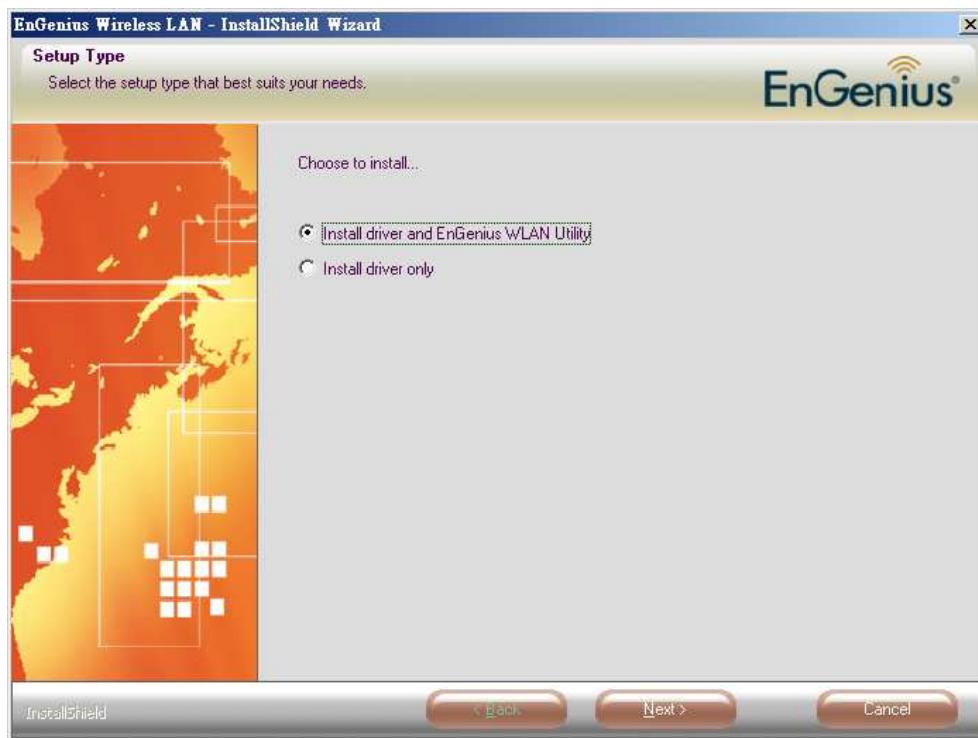
3. Once the setup begins you will see the **InstallShield Wizard**. Select **Install driver and EnGenius WLAN Utility** and then click on the **Next >** button.
