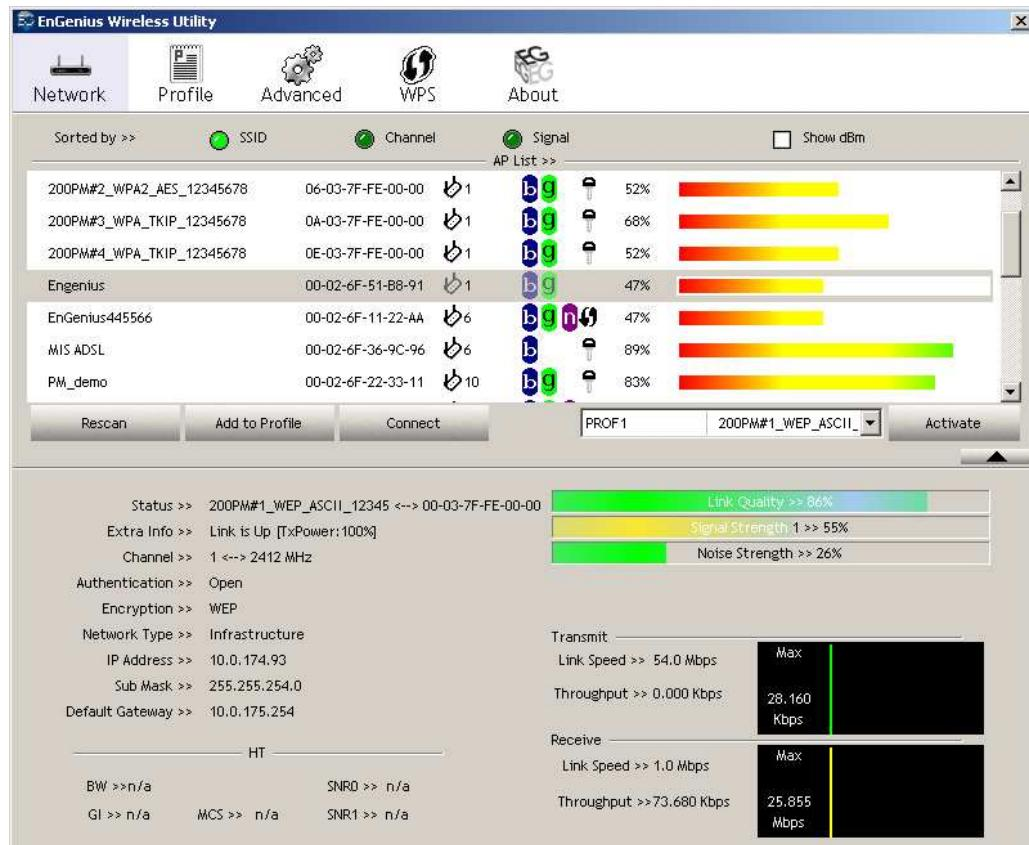
The information is displayed in the following order: SSID, MAC, Channel, Mode, Security, and Signal.
