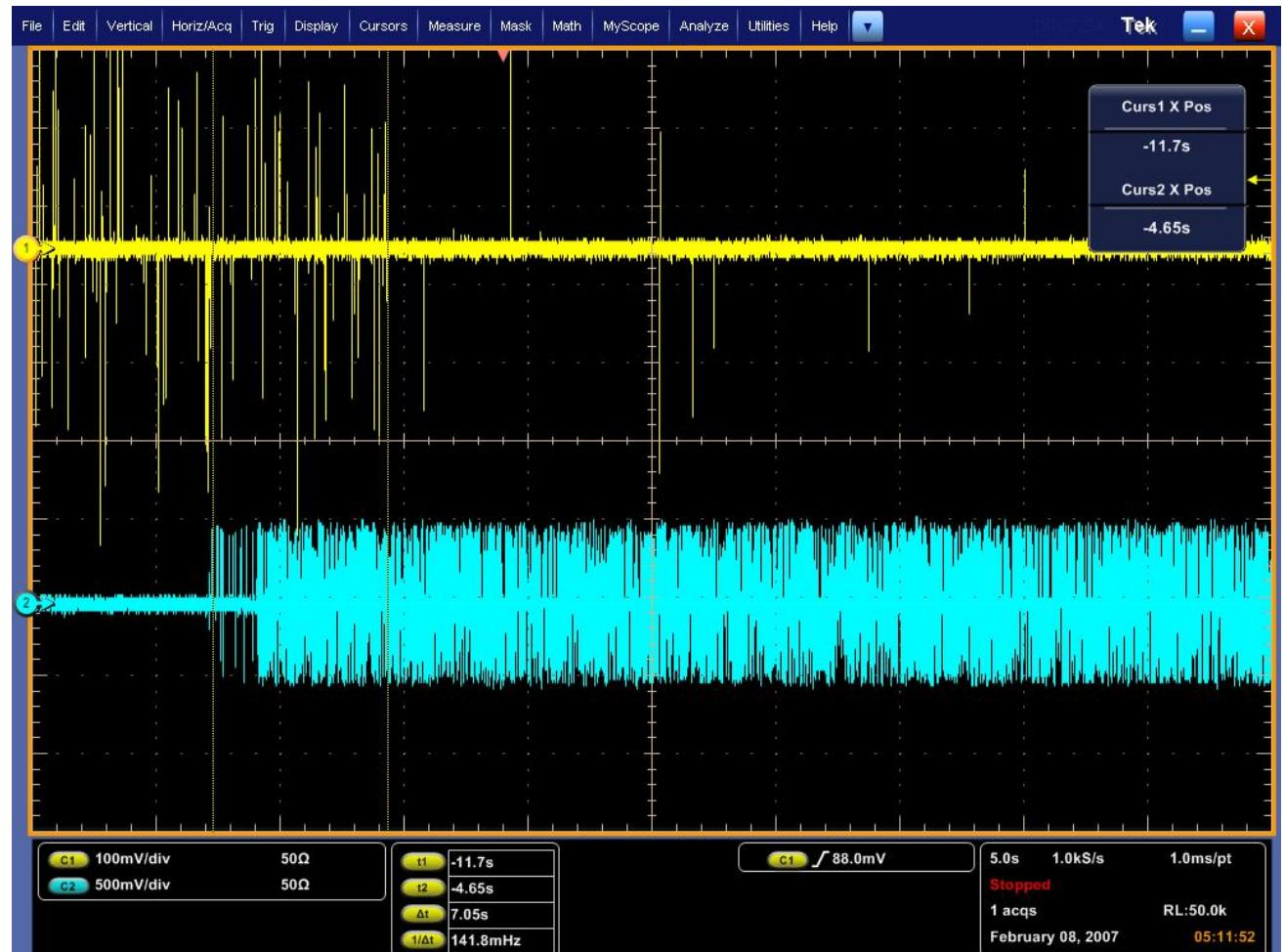
The yellow plot shows the output of the WLAN part , the light blue the output of the PCS part.
