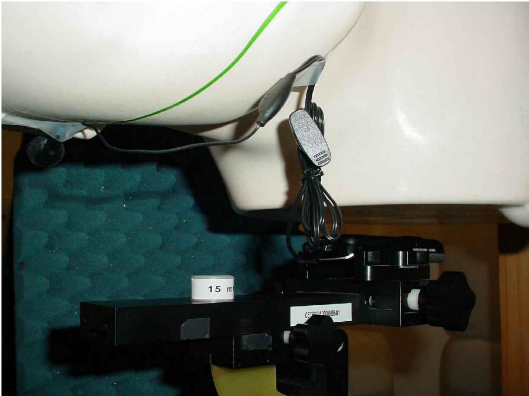
Photo 20: test position body worn rear side (15 mm distance)
